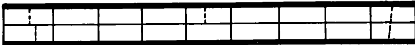
SECTION 2-C SHOWING ASSUMED CHANGE FOR REDUCTION OF CENTER THICKNESS, INCREASED EDGE THICKNESS AND INSTALLATION OF CENTER JOINT
