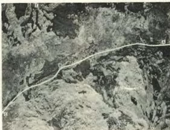
3.—RECONNAISSANCE ROUTE ALONG A RIDGE OUTLINED UPON A SINGLE PHOTOGRAPH BY STEREOSCOPIC PROCESSES
