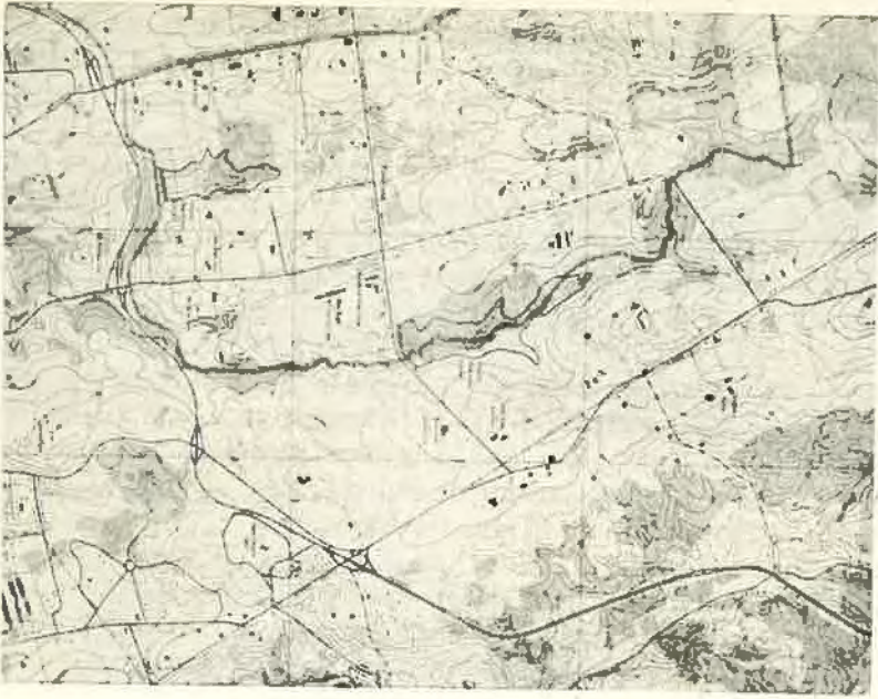
Figure 4. Topographic Map of a Section of Northeastern Hill Country Showing Highways With Both Spline and Long Tangent Alignment Intersecting at Grade Separation Lower Left Centre.
