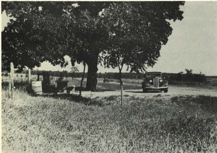
Figure 11. Small turnout southern Atlantic Plains region. Note permanent type of table and bench installation. Small areas of this type are usually provided with movable tables and benches so that areas can occasionally be "rested" to avoid serious damage to trees and turf by passage of vehicles over root systems.
