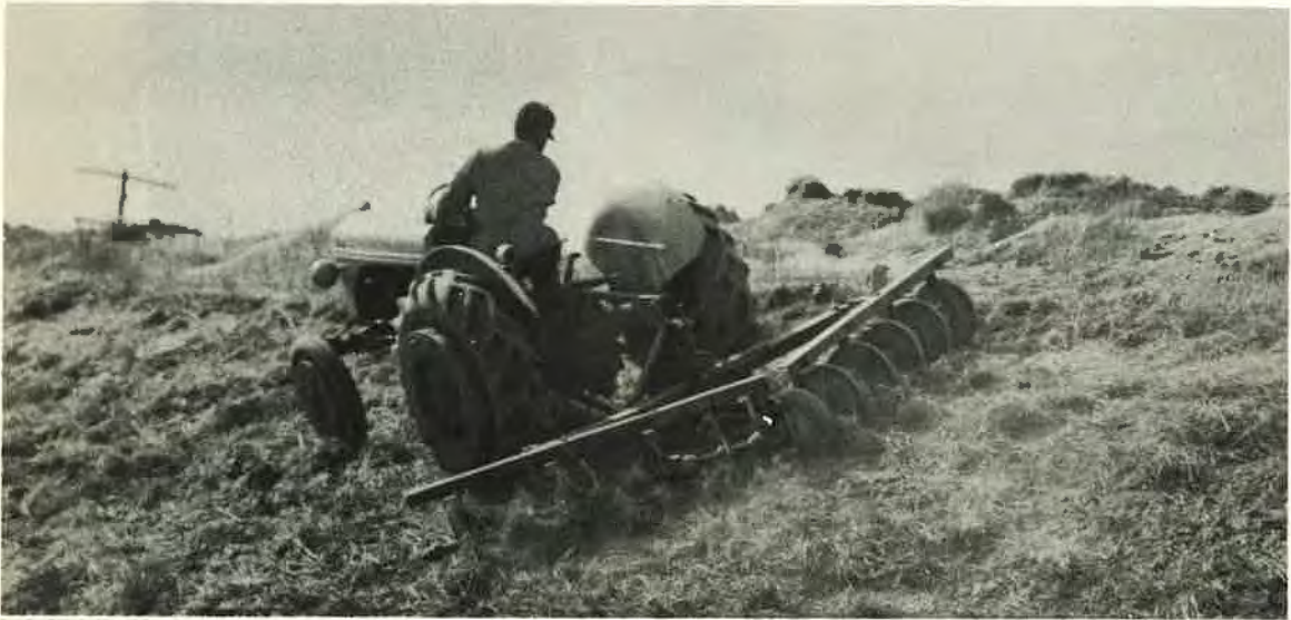
Disc - The disc has the alternate disc removed for stabilizing mulch. The machine can be set at various degrees to govern the depth of cutting.
