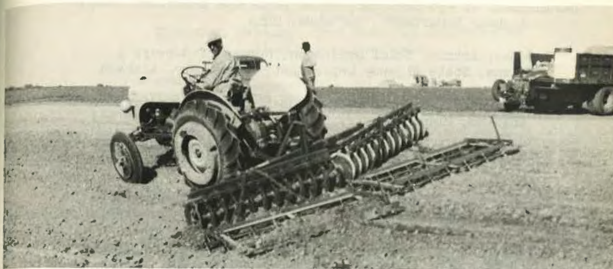
Spike-Tooth Harrow - One or more sections can be used. A lever controls the angle of the cutting teeth so various depths of soil can be loosened.
