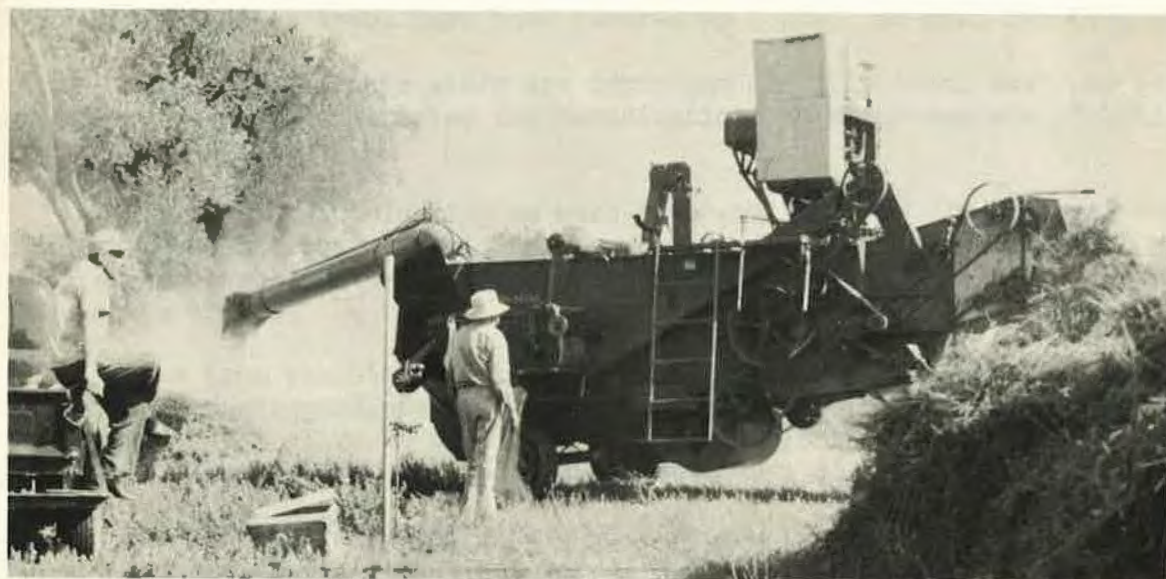
Threshing Machine - The machine is powered by a pulley which is driven by belt attached to auxiliary power such as a tractor, truck, or Jeep. The machine is mounted on rubber tires and is easily towed. The material to be threshed is placed in the machine which separates the seed from the straw by a series of knives or beaters and various screens moving in such a manner to give a sifting effect.
