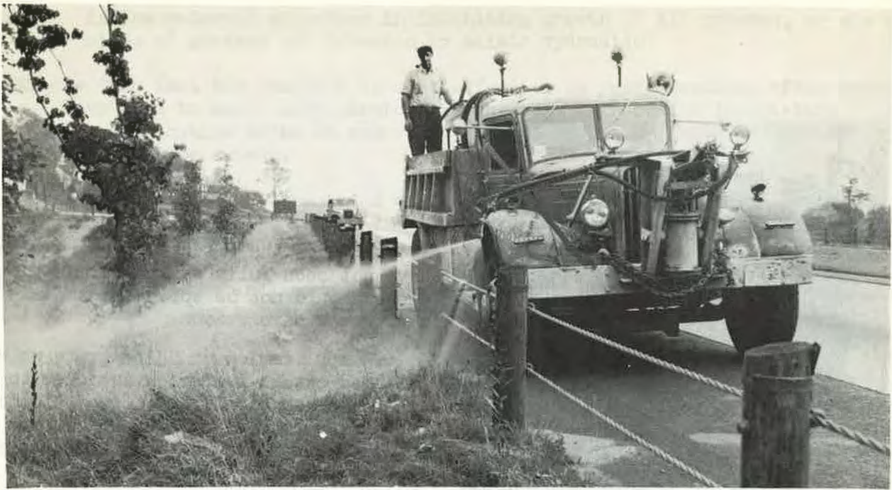
Figure 2. Spraying MH on roadside areas at 200 lb. pressure, delivering 50 gal. of liquid per acre at 10 mph.
