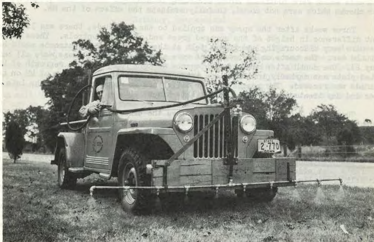
Figure 1. Spraying MH on the esplanade at 50 lb. pressure, 40 gal. of liquid delivered at 5 mph.
