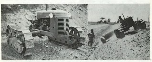
Tractor - This tractor is engineered and built for mobility and compactness for swift maneuvering and extra stability to work safely on hillsides. The tread width range is 60 and 68 in.
