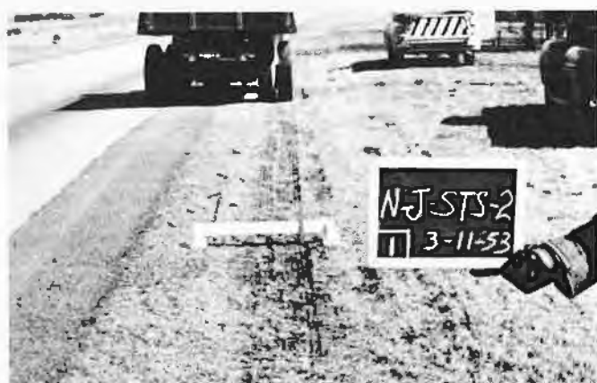
Fig. 1. Test equipment after one pass on test Area 2. Rigid bridge and graduated scale in position to measure penetration. Loaded truck in background.
