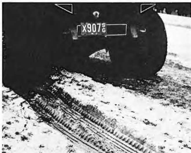
Fig. 6. Loaded truck leaving test area NJ-STS-8 and reentering stabilized turf shoulder.
