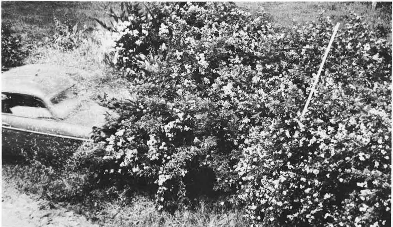
Figure 4. The car just entering the Rosa multiflora Hedge, Traveling at 47 mph., the vehicle was stopped in 20 feet without injury or discomfort to occupants. (Connecticut State Police Photo furnished through courtesy of C. R. Burr & Co., Inc.)
