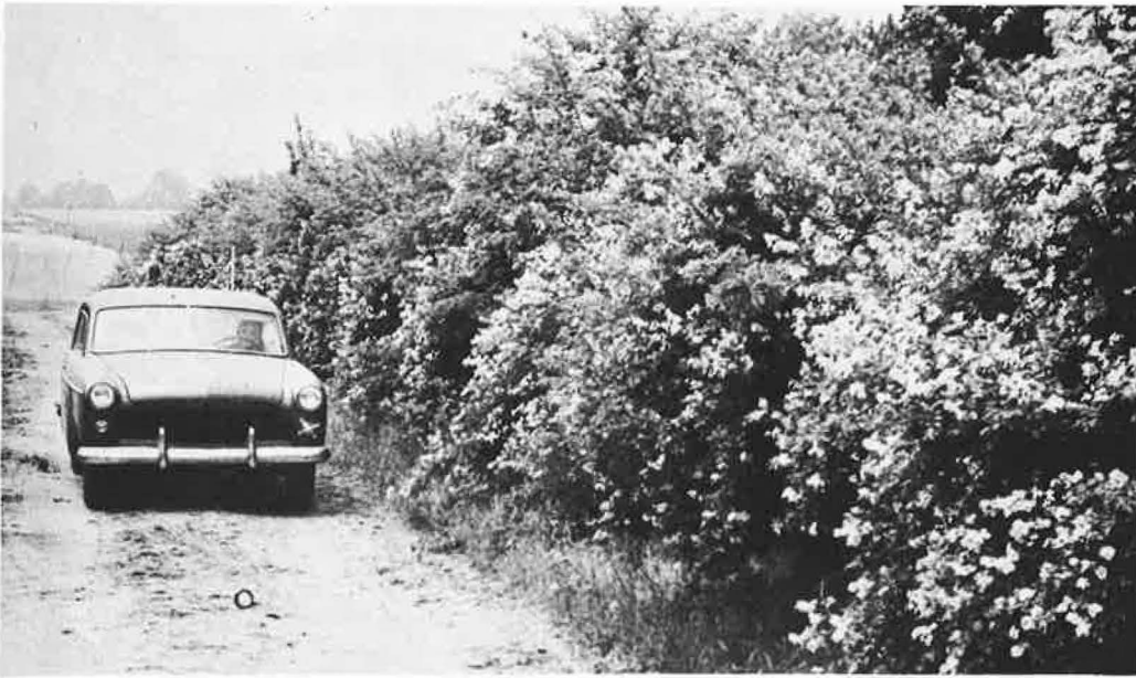
Figure 3. A Rosa multiflora hedge which was used in crash tests. The car used in the tests is the stock model Aero-Willys. (Connecticut State Police Photo furnished through courtesy of C. R. Burr & Co., Inc.)
