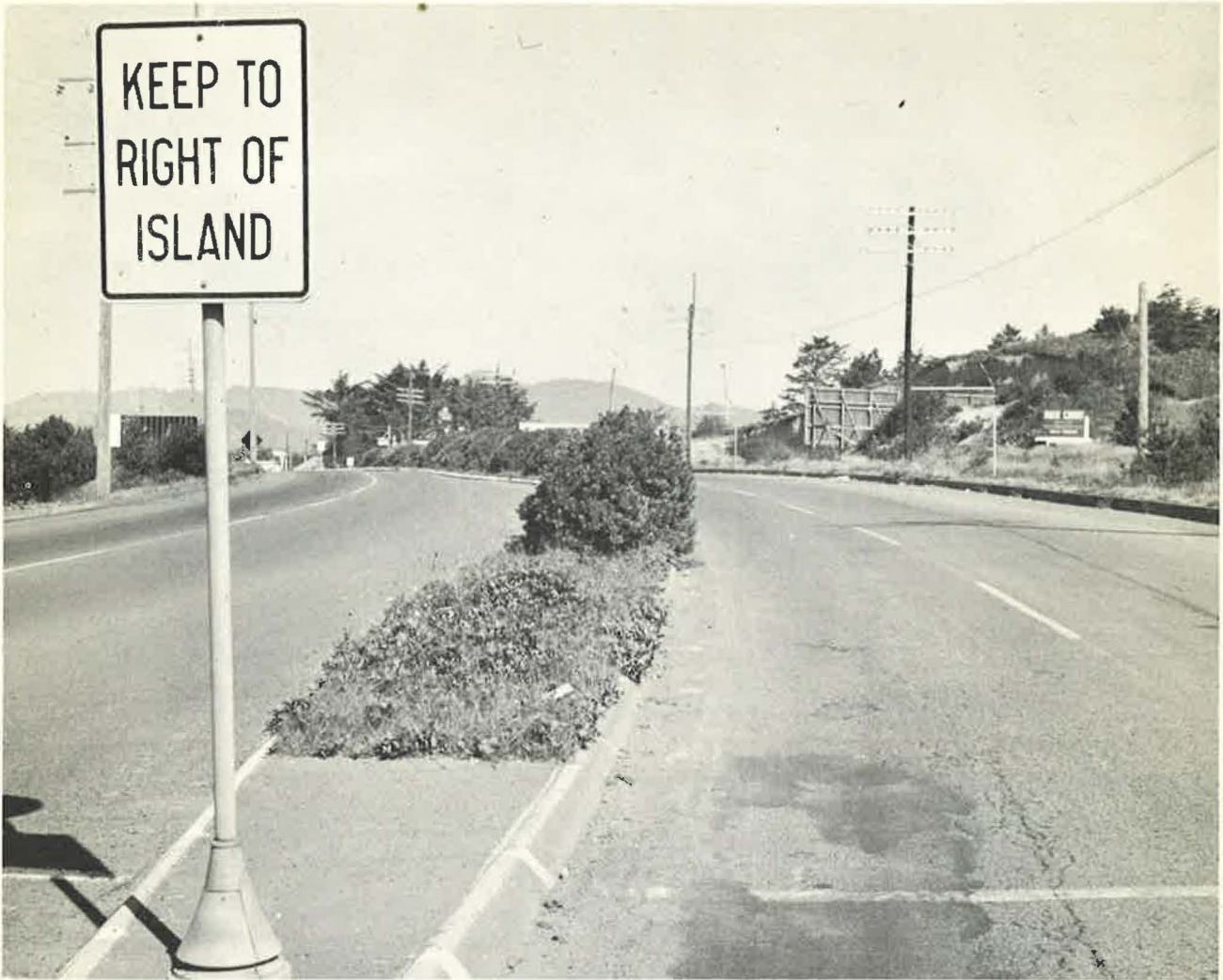
Figure 16. Planting at Oceanlake, Ore., of native materials: Pacific waxmyrtle ( Myrica californica ), hairy manzanita ( Arctostaphylos columbiana ), salal ( Gaultheria shallon ), and a few shore pines ( Pinus contorta ). This median island, planted in 1946, has proved effective as a traffic delineator and has eliminated headlight glare. The width of the island varies from 5 to 20 feet. (Courtesy Oregon State Highway Department)
