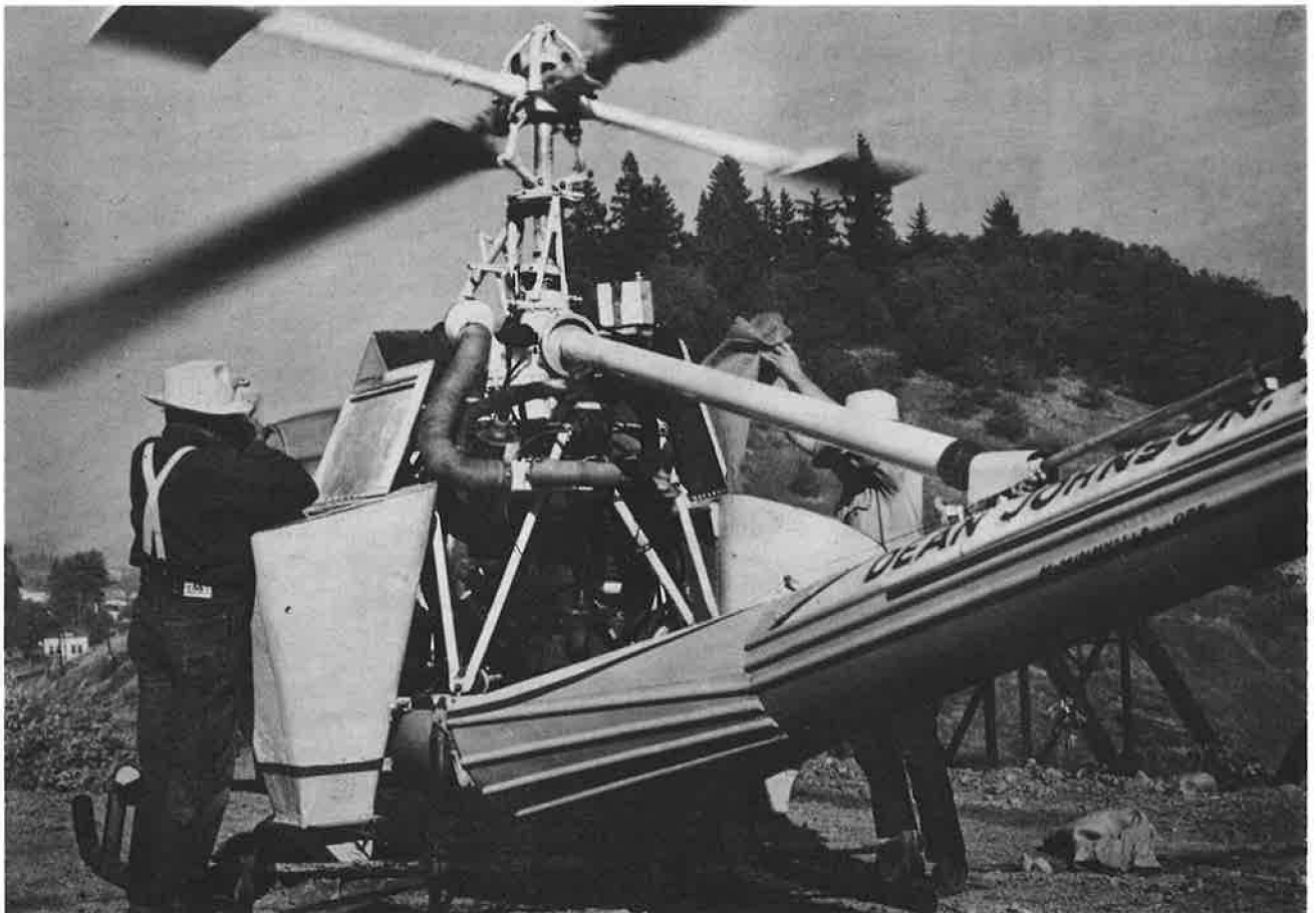
Figure 1. View shows helicopter being loaded with grass seed. Each hopper contained approximately 126 lb, enough for about 8 acres per load.
