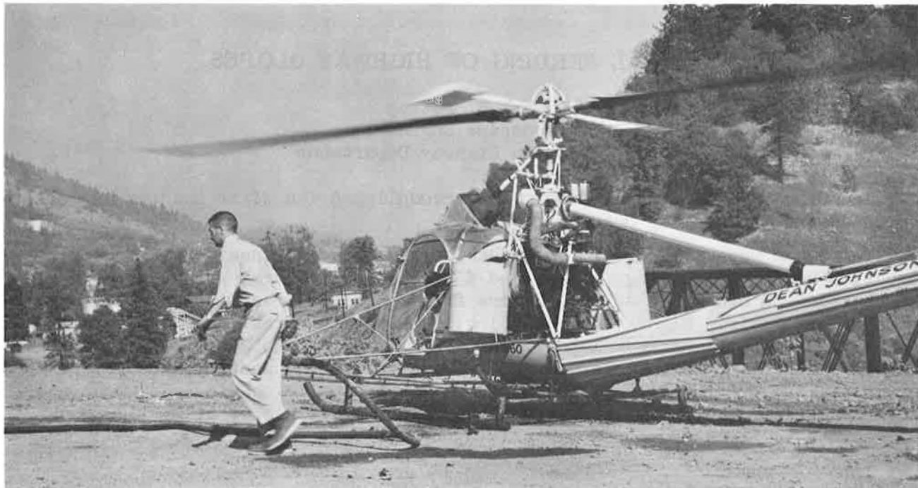
Figure 2. Completing the reloading of the helicopter with liquid fertilizer. The two barrels hold a maximum of 30 gallons each.
