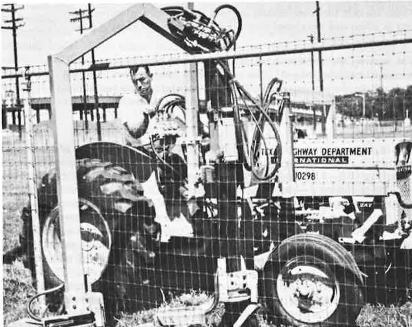
Figure 2. The new "Rail Bird" mower designed for guardrail mowing. (Photo courtesy of TEXAS HIGHWAYS.)
