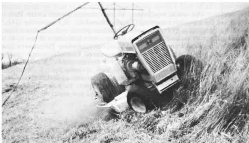
Figure 4. This is a pilot model of a mower that can be remotely-controlled by either radio or guide cable. It is being developed at the University of Illinois. (Photo courtesy of University of Illinois.)
