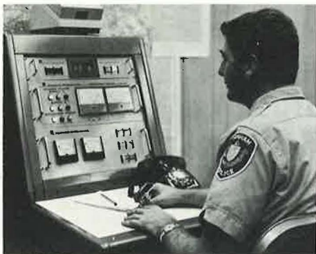
Figure 2. Dual receiving station at central headquarters—such as a police station—has a visual readout that indicates the number of the box sending the distress signal, and a visual indicator that describes the reported emergency's nature. It also provides a tone alert that calls the operator's attention to a received message.
