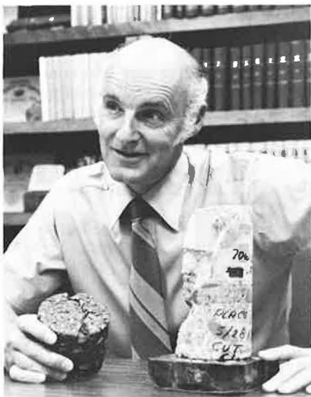
Roger V. LeClerc, Materials Engineer for the Washington State Highway Commission, holds an asphalt core from one of the early thick-lift sections and a portland cement core from one of the joint study sections. Plastic tape being evaluated for joint sealing can be seen at the top of the PCC core.
