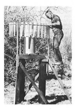
A precipitation gauge is placed in a sheltered spot for accurate recording. Baffles break up wind currents around the gauge.
