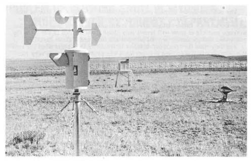
Some of the instruments used to collect weather data are shown here. Mounted on the pole is an instrument cluster consisting of an anemometer, wind vane, and thermometer to record wind velocity, wind direction, and temperature. In the center of the photograph is a station containing a pyrheliometer for recording solar radiation, and at the far right is the blowing snow gauge that measures the amount of snow blown by the wind.
