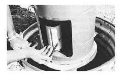
A precipitation gauge under the blowing snow recorder measures the amount of snow driven by the wind. It is easily removed for checking and maintenance.
