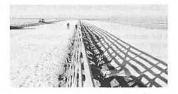
Snow expert Ronald D. Tabler checks the anchorage on a portion of the snow fence used as a test section at Cooper Cove, Wyoming.
