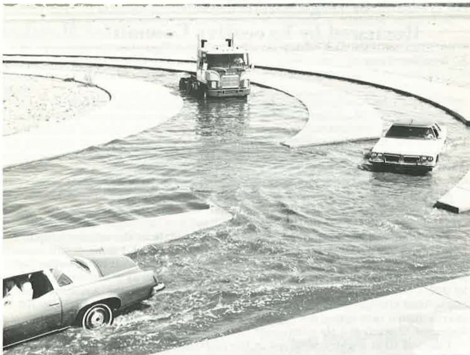
A novel feature of the General Motors Desert Proving Ground is this water facility, which has many applications in checking vehicle handling, waterproofing, and related subjects.
