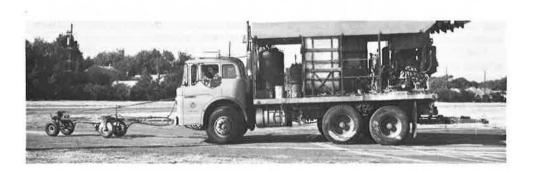
Personnel requirements for traffic striping may be decreased 50 percent. Convenience to public traffic is greatly enhanced. California Highway Maintenance Work Standard for placing median barrier stripe using the conventional cold paint system is 3.7 man-hours per mile of stripe. Using the hot paint system, it is estimated that the labor requirement may be reduced to 0.6 manhour per mile.
