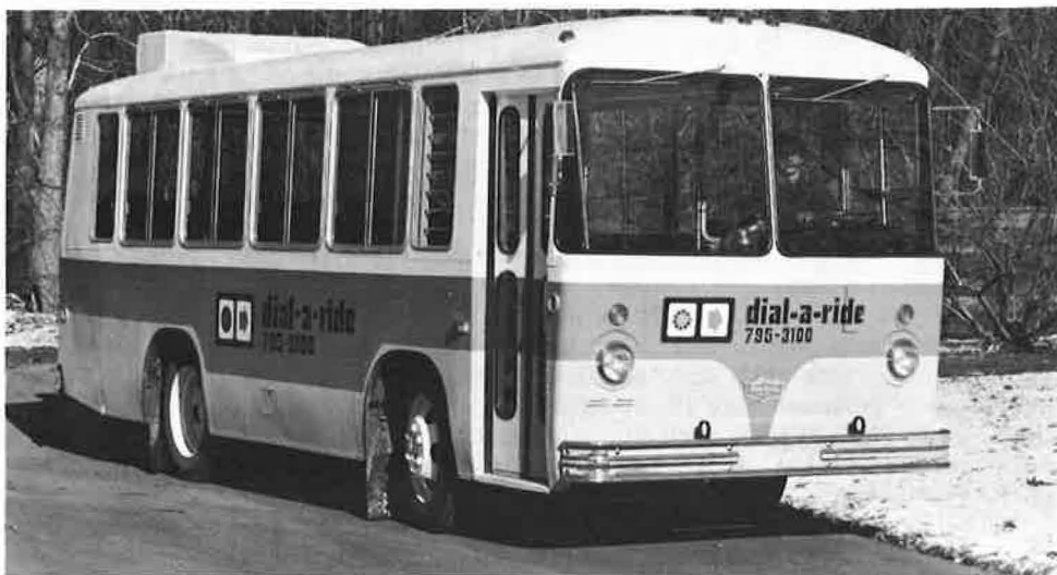
Seventeen-seat bus is typical of the 12 operating in the Haddonfield demand-actuated system. All buses are radio-equipped and were supplied by the Twin Coach Company of Kent, Ohio.
