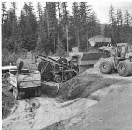
Figure 1. Portable emulsified asphalt mix plant.
