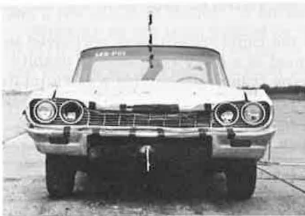
Damage to the front of the test automobile was minimal even after crashing into the rear of the attenuator at 60 miles per hour.
