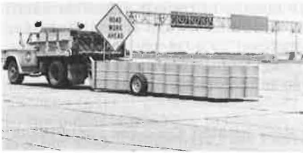
The crash cushion trailer, consisting of 30 barrels welded together and mounted on a single axle, is shown before testing at the Texas Transportation Institute facility.
