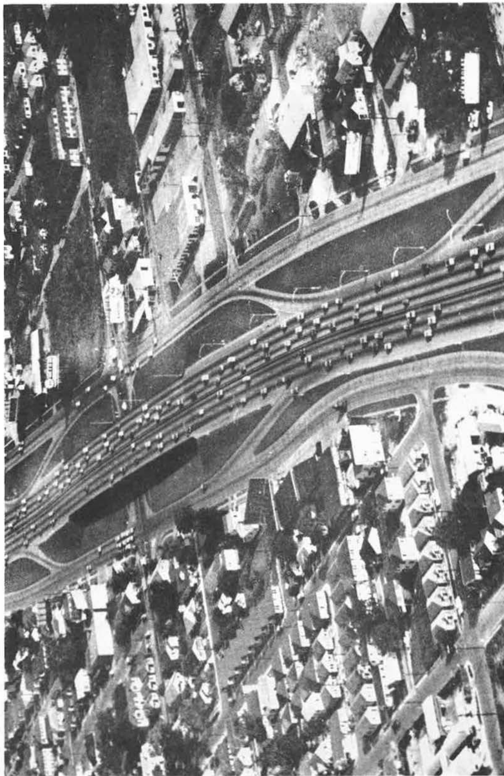
Figure 14. Conventional two-level diamond interchange.
