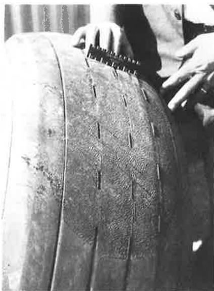
MAIN LANDING GEAR TIRE WITH REVERTED RUBBER SKID PATCH
