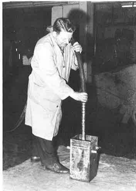
Figure 4. Complete compaction of loosely charged concrete by a vibrator centrally inserted into the container (also possible by intensive tamping).
