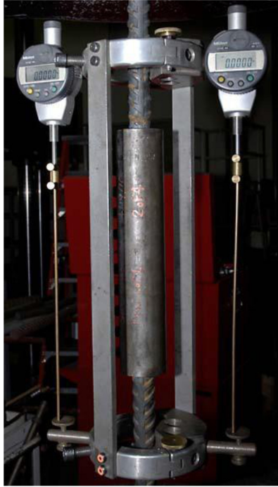
(a) Device with dial indicators (California Test 670)
