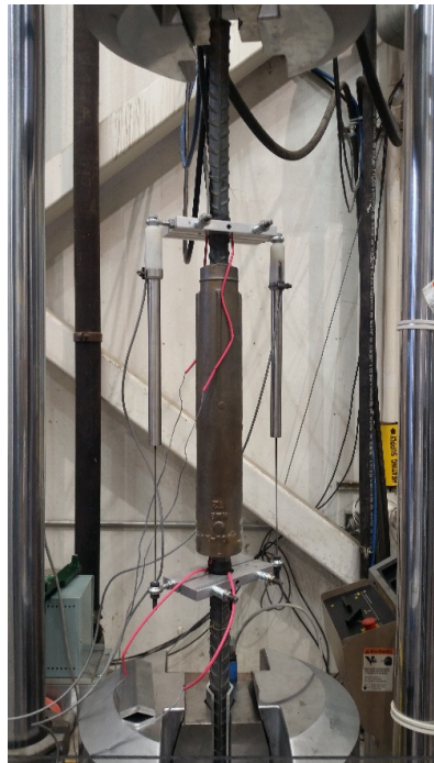
(c) Device with two LVDTs
