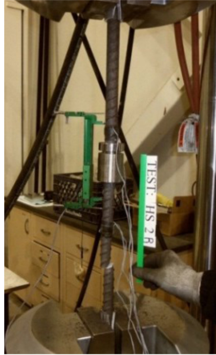
(b) Device with extensometer
