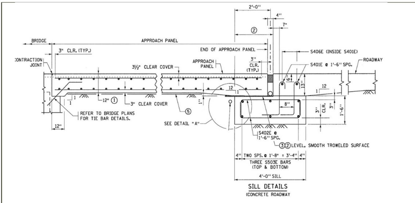
**Figure 67 MnDOT Approach Slab Connections**
