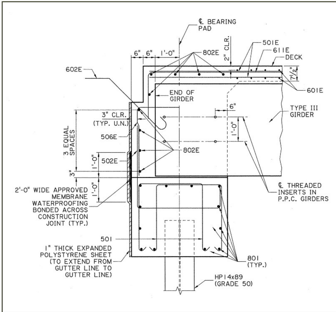
**Figure 40 LaDOTD Integral Abutment**
