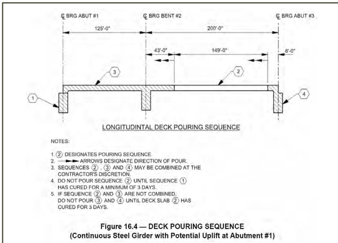
*Figure 29 UDOT Deck Pouring Sequence (Continuous Steel Girder with Potential Uplift)
