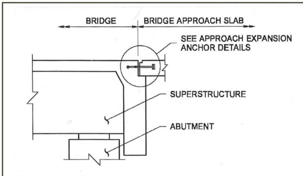
Figure 34 Semi- Integral Abutment (courtesy WSDOT)
