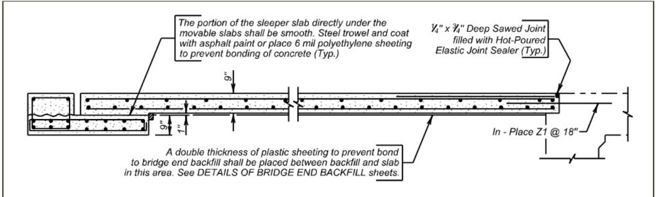
**Figure 69 SDDOT Approach Slab**
