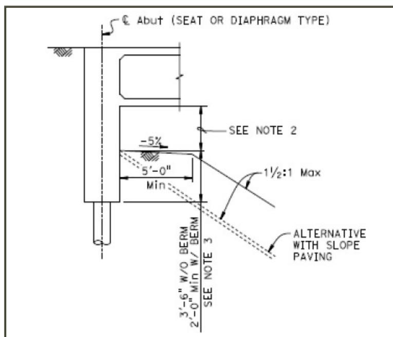
Figure 51 Caltrans Abutment on Piles without Footing
