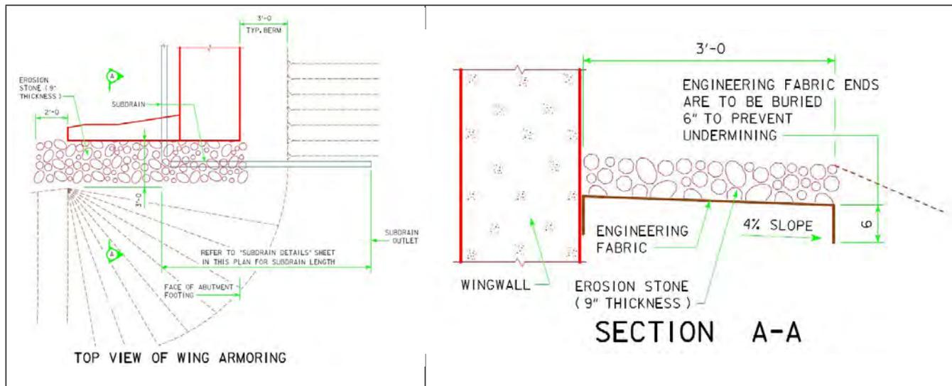
**Figure 48 Iowa DOT Wing Armoring**
