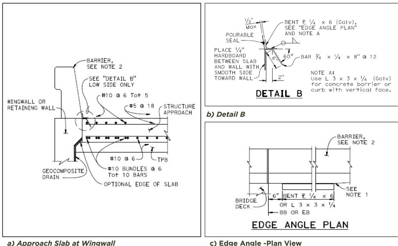
Figure 63 Caltrans Expansion at Shoulder (Caltrans Standard Plan B9-5)
