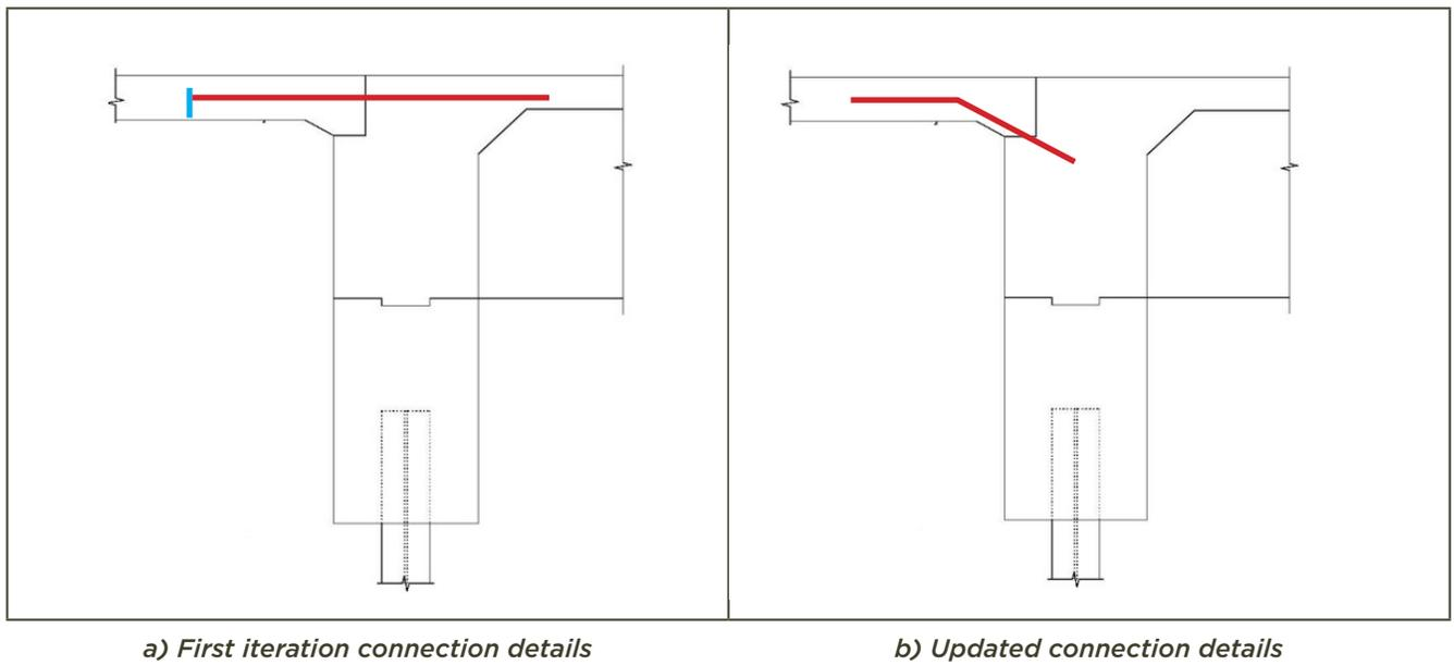
**Figure 15 MnDOT Approach Panel Connection Details**
