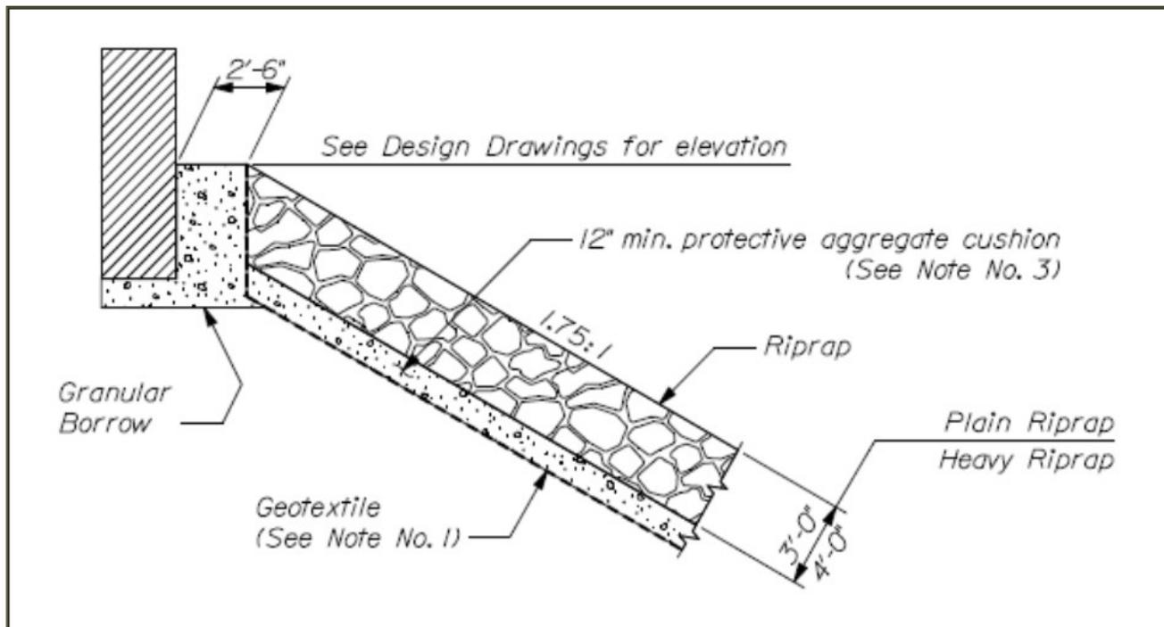
**Figure 49 MaineDOT Riprap Slope Integral Abutment**
