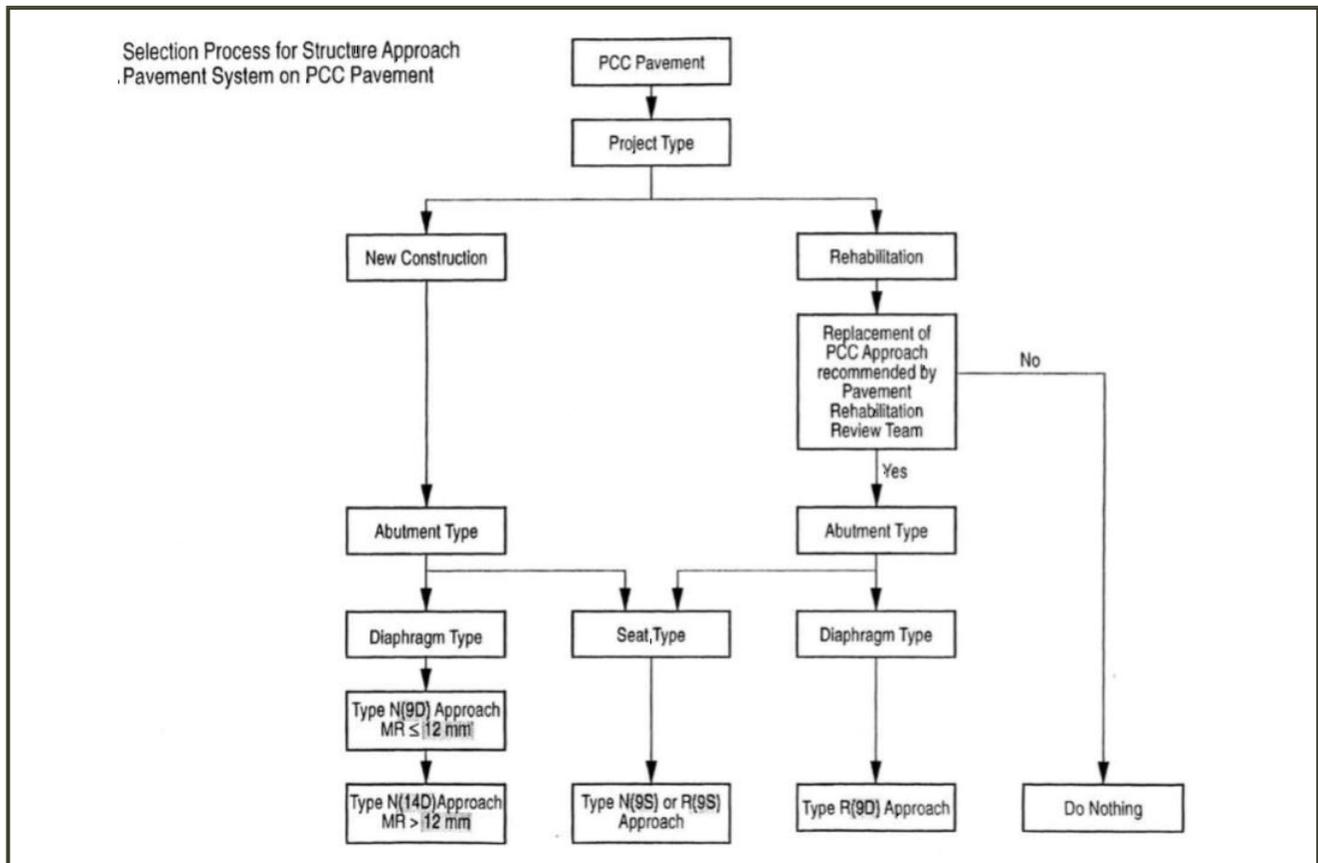
**Figure 16 Caltrans Approach Pavement Selection Process (3)**
