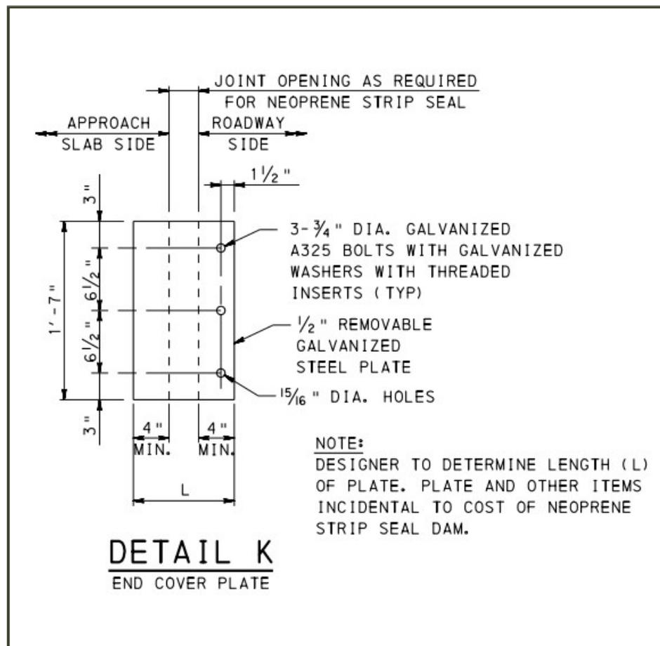
Figure 64 PennDOT End Cover Plate Detail (BD-628, sheet 20, Detail K)
