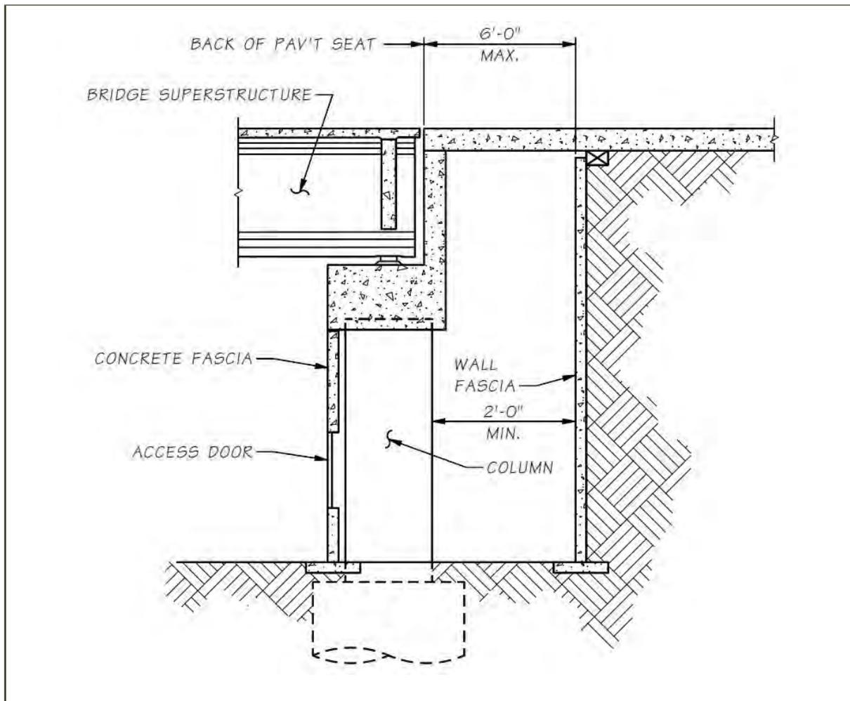
Figure 100 WSDOT Isolated Bent-Type Abutment (BDM Fig. 7.5.1-4)
