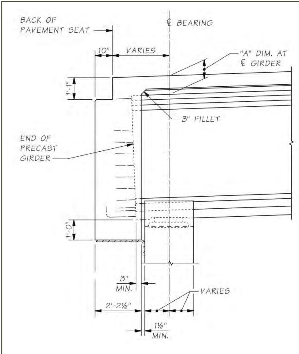
Figure 61 WSDOT End Diaphragm on Girder (BDM Fig. 5.6.2-3)
