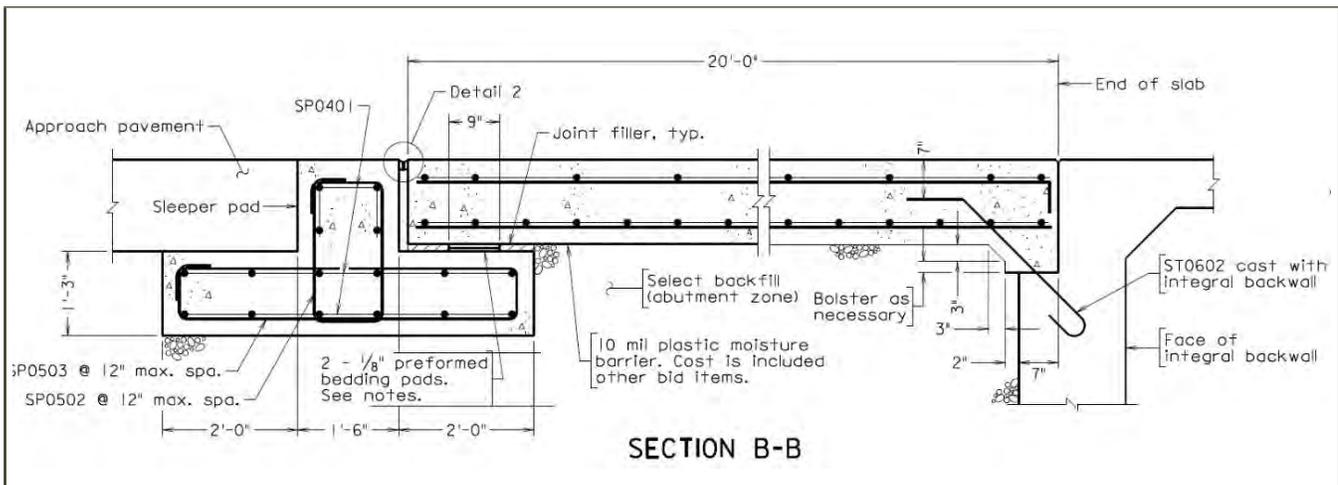
Figure 71 VDOT Approach Slabs for Integral and Semi-Integral Abutments
