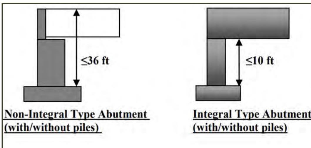
**Figure 22 Caltrans Wall Heights per Abutment Types**
