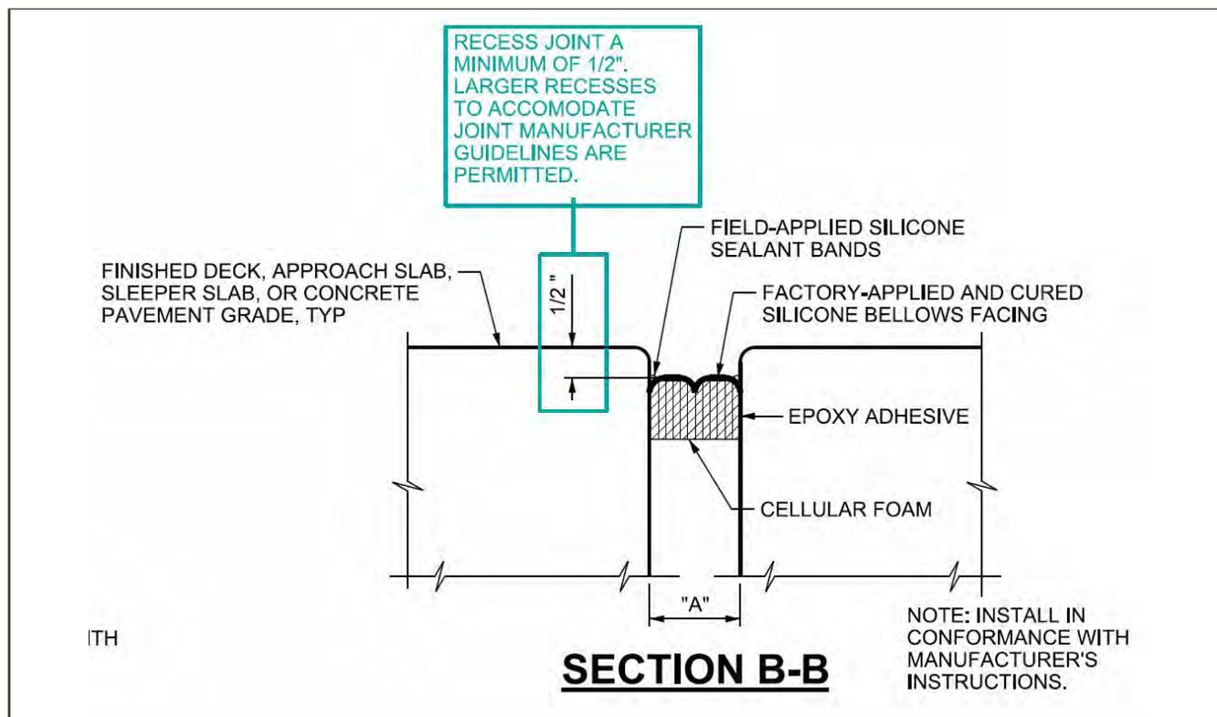
Figure 81 UDOT Compression Joint Seal Type A
