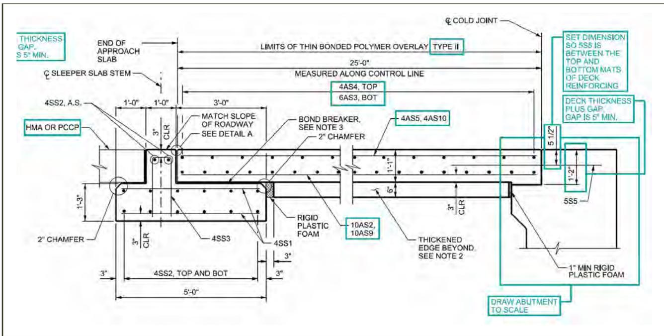
Figure 85 UDOT Sleeper Slab Details
