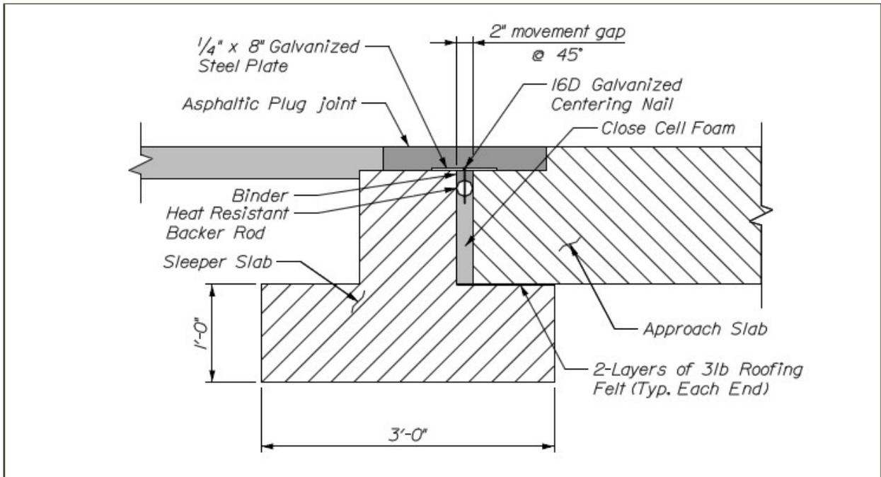
**Figure 84 MaineDOT Typical Sleeper Slab Detail (5)**
