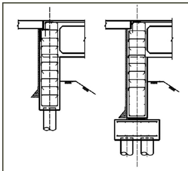
Figure 38 Caltrans Integral (Diaphragm) Abutment
