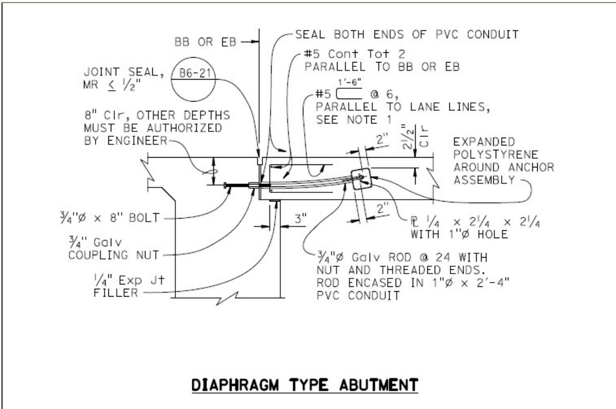
Figure 66 Caltrans Structure Approach Type N (30) (Standard Plan B9-1)
