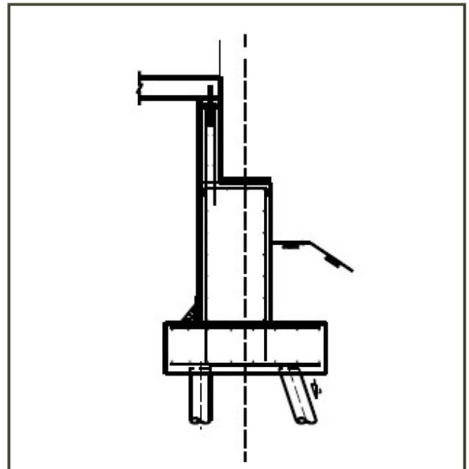
Figure 37 Seat Abutment (Courtesy of Caltrans)
