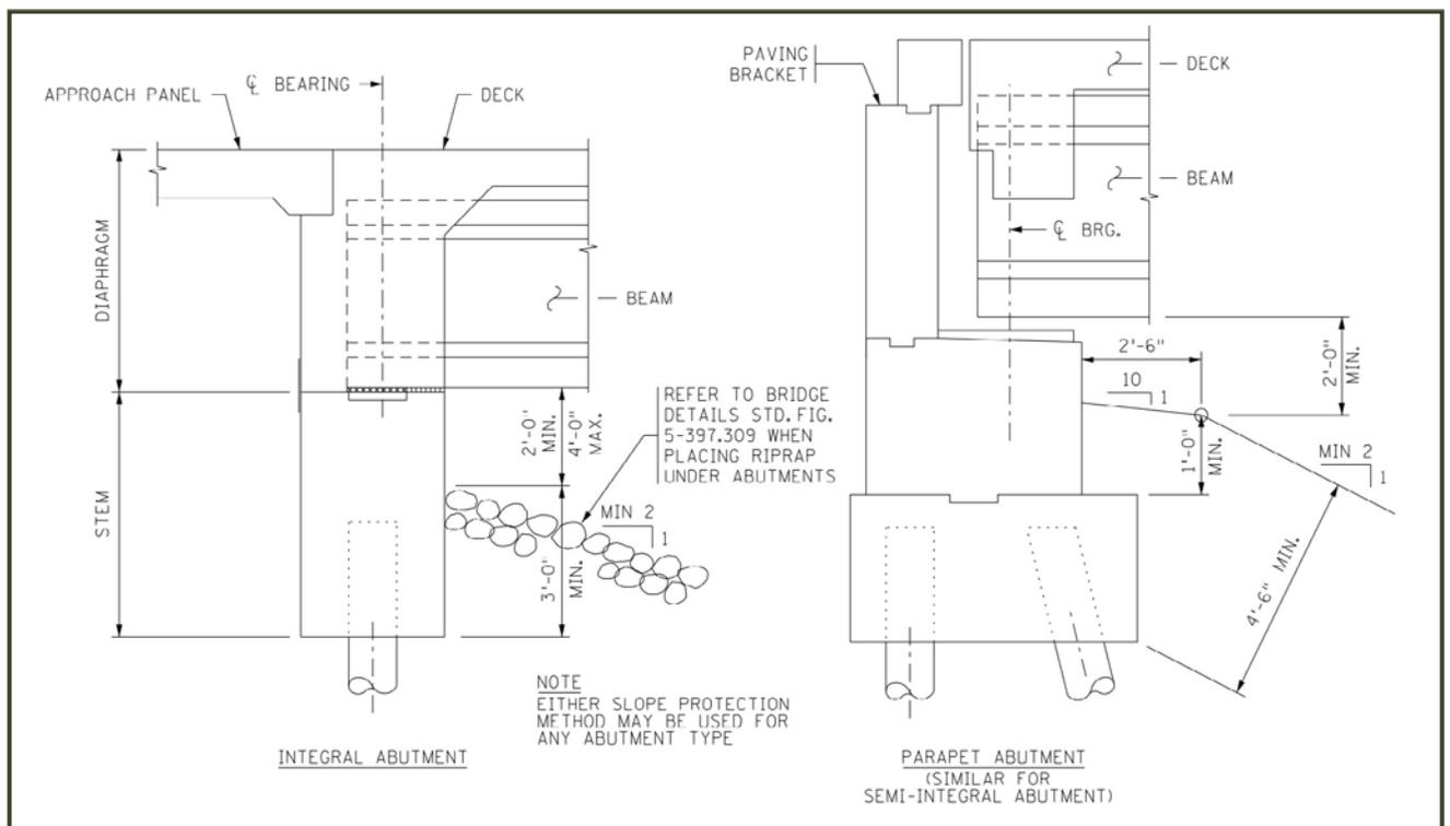
Figure 17 MndOT Cover and Clearance Requirements (MndOT Design Manual Figure 11.1.2)
