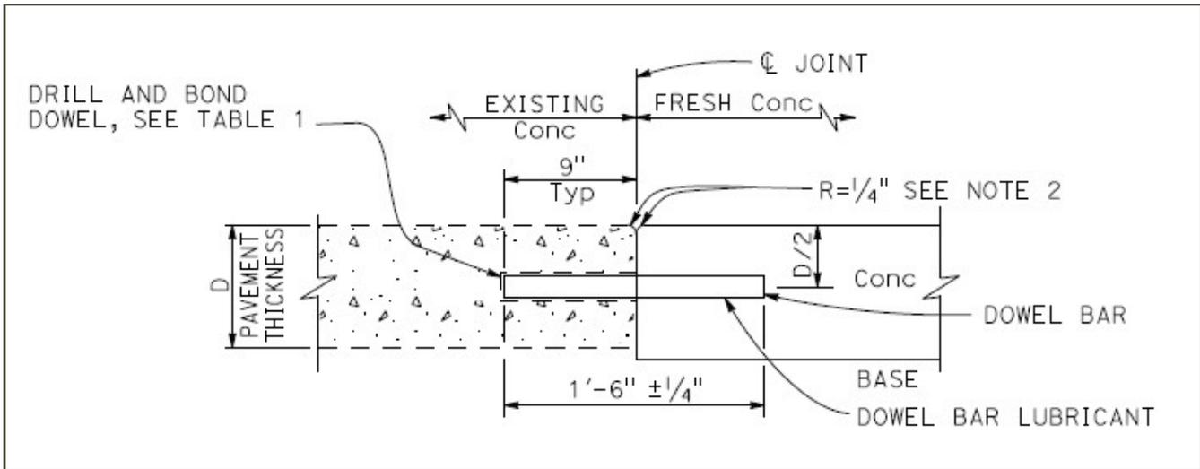
**Figure 74 Caltrans Transverse Construction Joint at Existing Pavement (Caltrans Standard Plan P10)**
