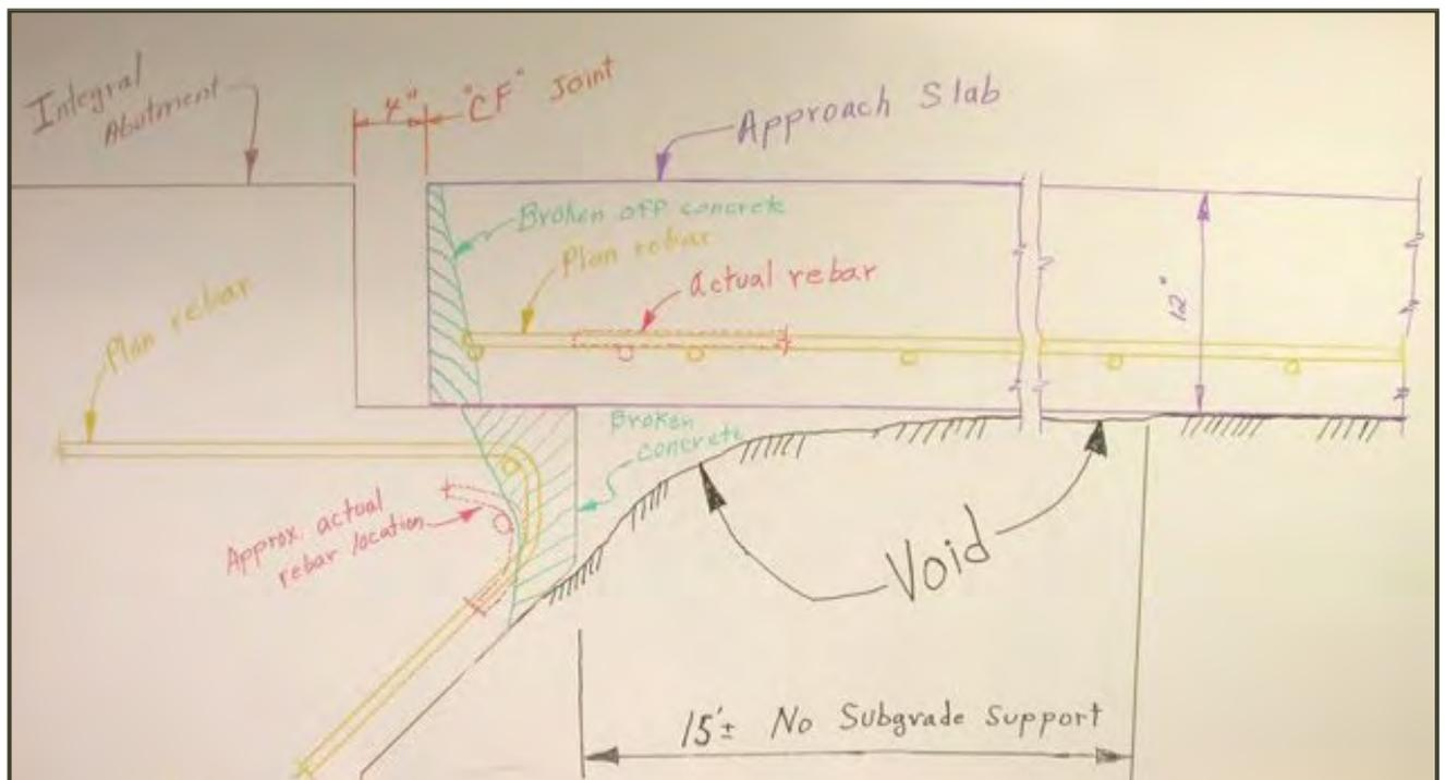
Figure 14 Iowa DOT Discontinued Detail - Broken Seat
