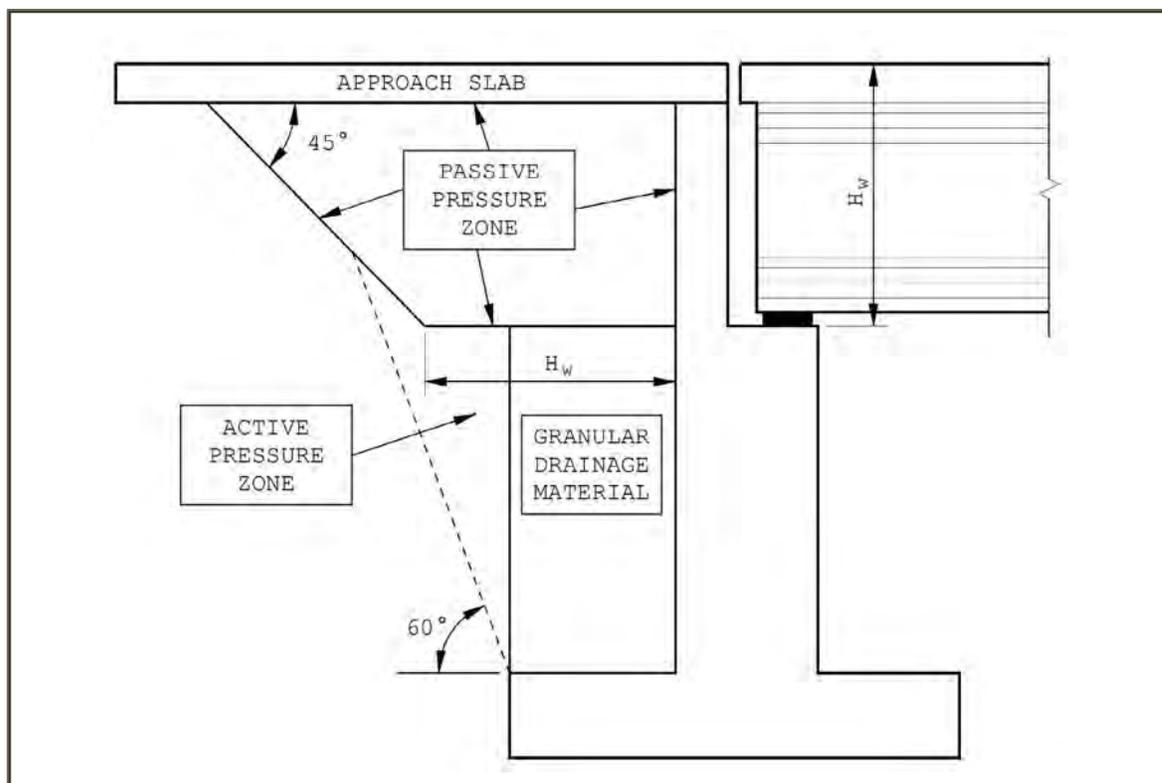
Figure 27 WSDOT L-Shape Abutment Backwall Does Not Fuse (WSDOT BDM Figure 4.2.11-1B)
