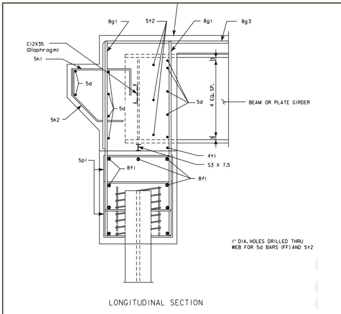
Figure 56 Iowa DOT Integral Abutment Section for a Steel Girder Bridge (Iowa DOT BDM)
