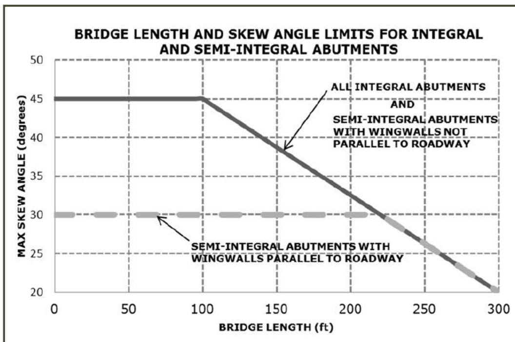
Figure 20 MnDOT Abutment Type Selection Chart (MnDOT BDM Figure 11.1.1)
