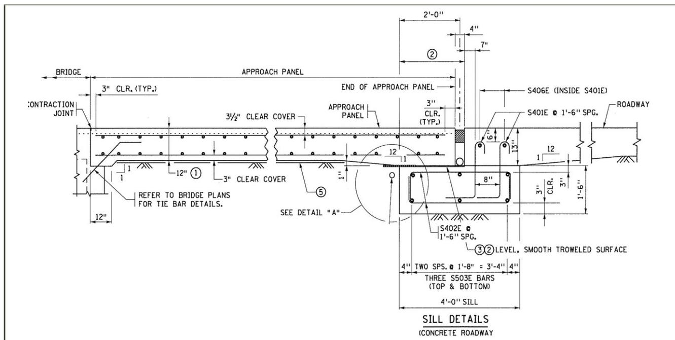
**Figure 77 MnDOT Approach Slab and Connection Details**
