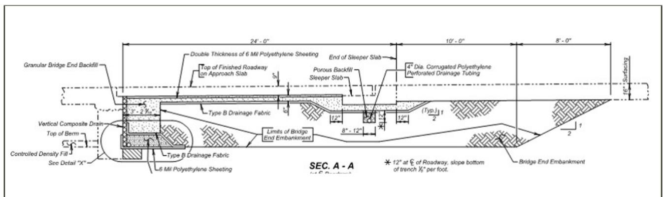
Figure 90 SDDOT Granular Bridge End Backfill
