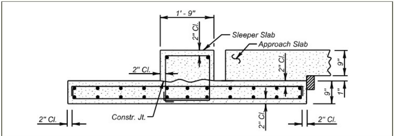
Figure 79 SDDOT Sleeper Slab for Concrete Pavement
