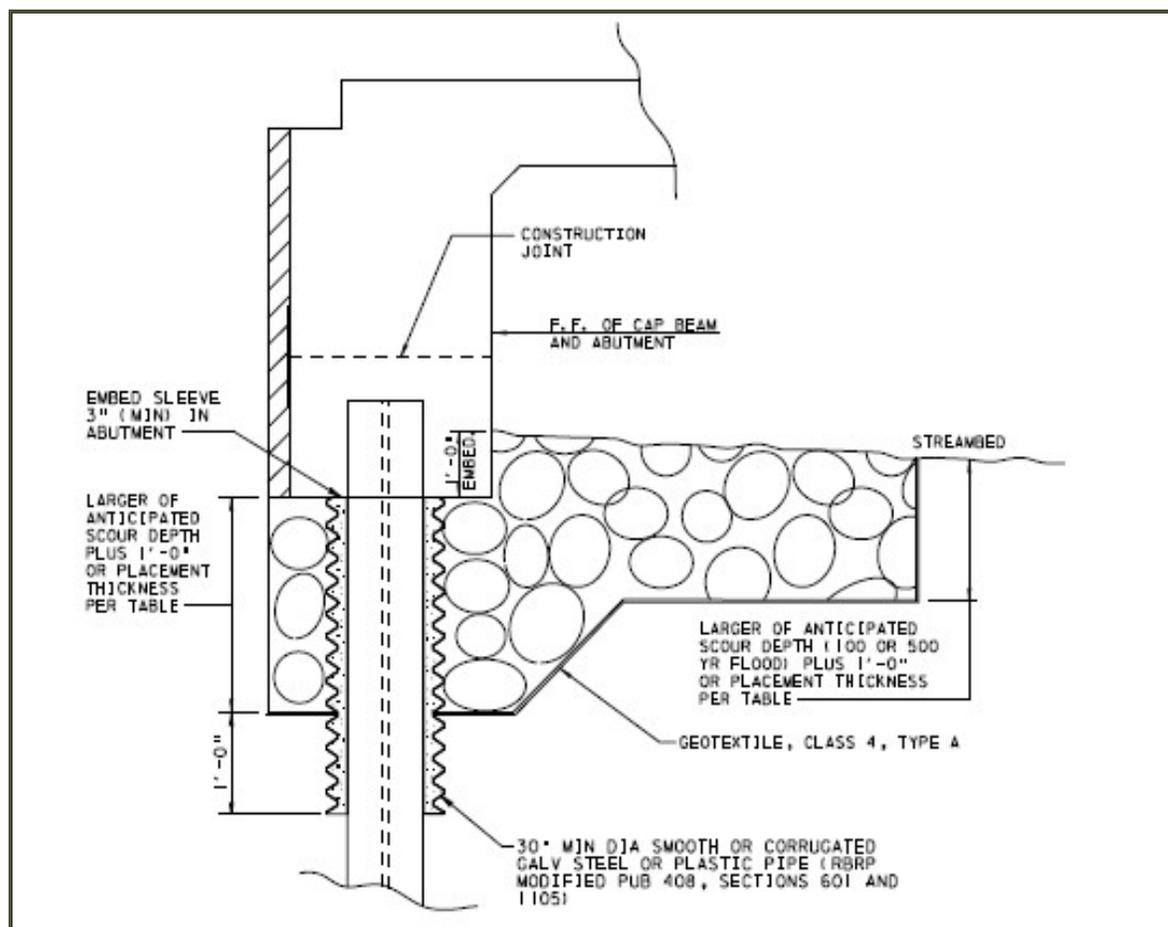
Figure 52 PennDOT Alternate Scour Protection Detail
