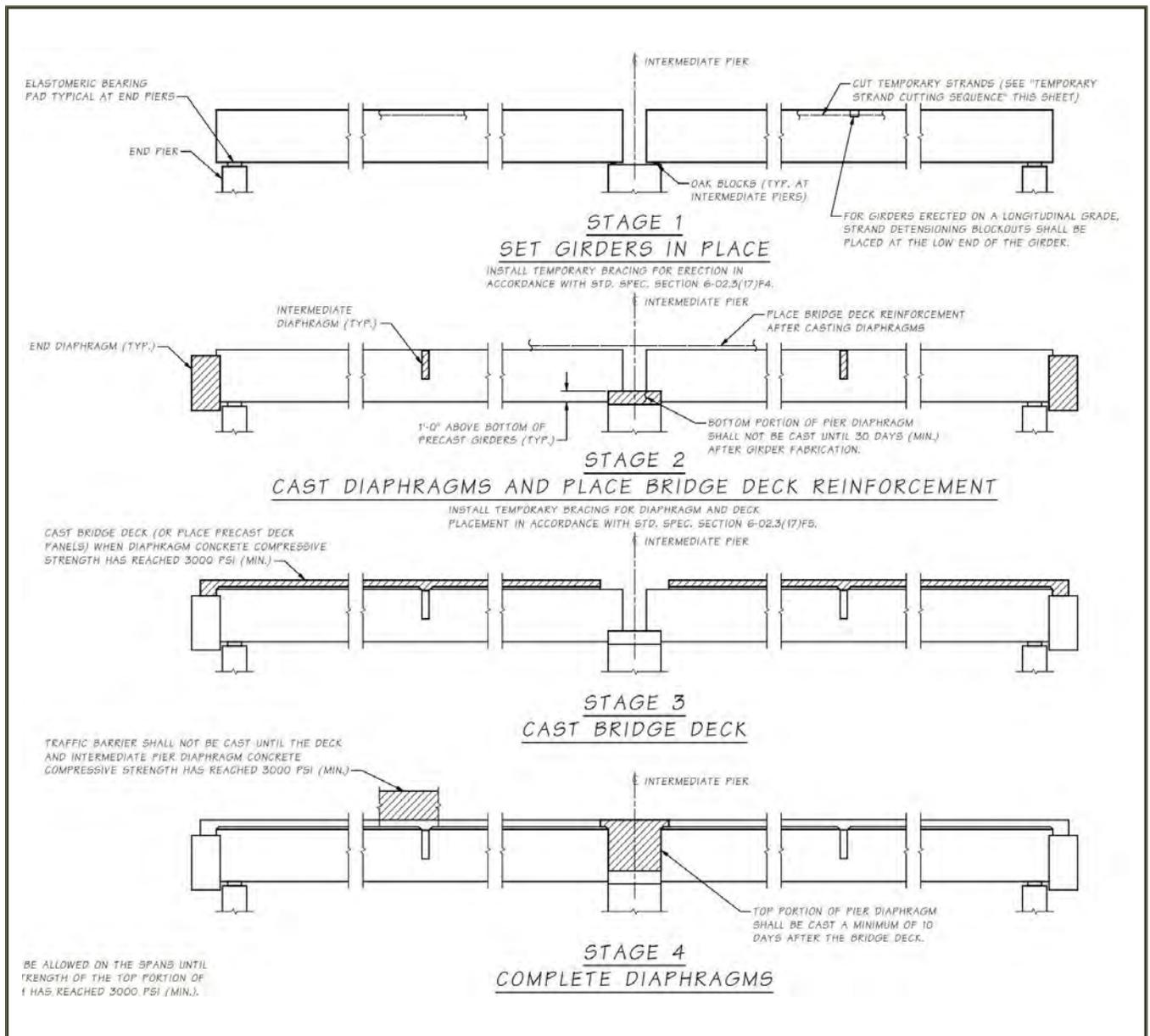
Figure 31 WSDOT Multiple Span Prestressed Girder Construction Sequence (WSDOT BSD 5.6-A2-2)
