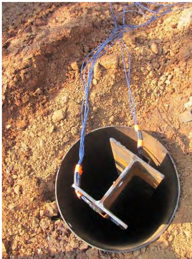
b) Pile Strain Gauges
