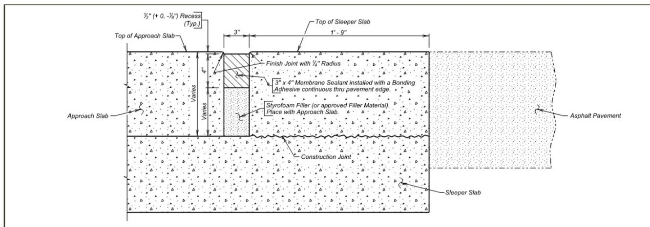
**Figure 78 SDDOT Sleeper Slab to Asphalt Transition**
