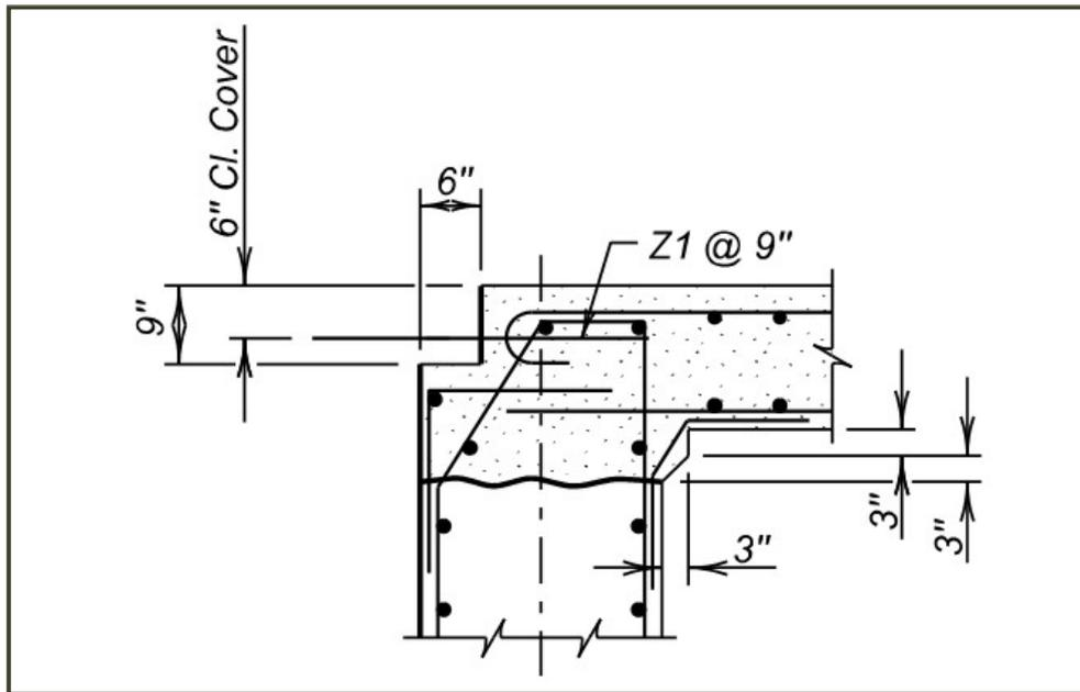
Figure 59 SDDOT Continuous Concrete Bridge Abutment to Bridge Deck Details
