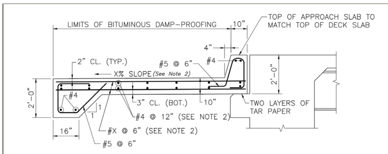
**Figure 82 MassDOT Approach Slab Details (MassDOT Drawing Number 3.1.14)**
