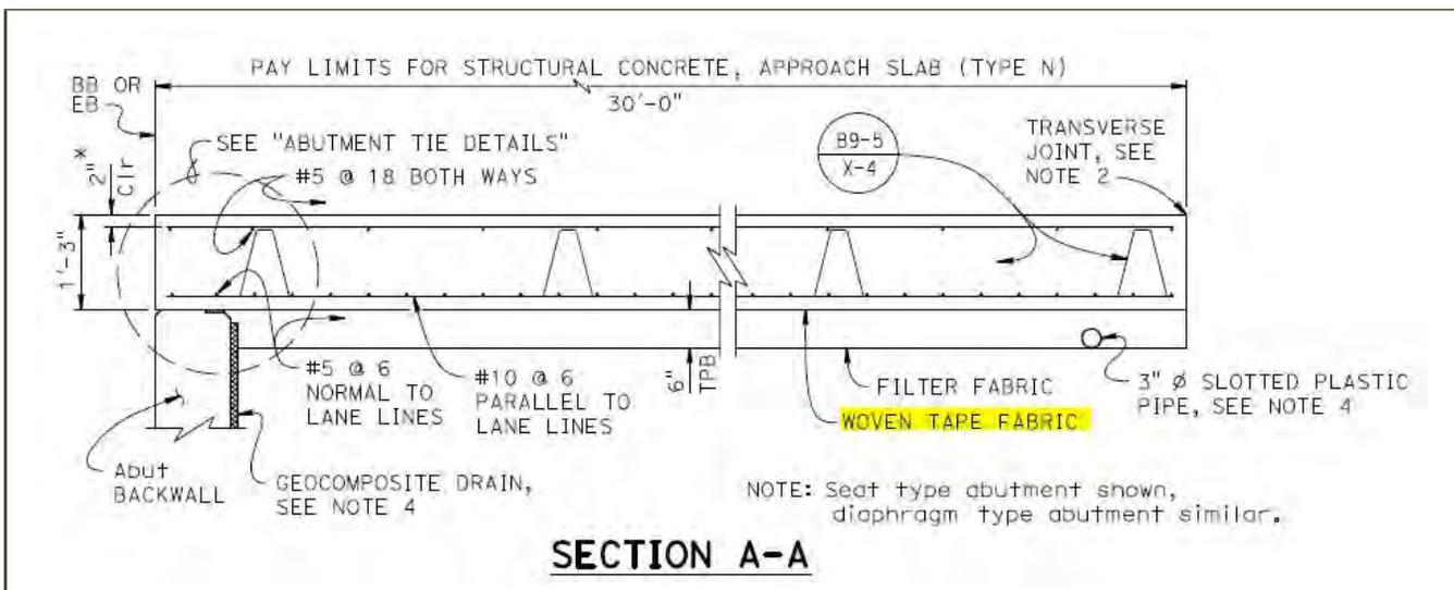
Figure 86 Caltrans Embankment Separator (Caltrans Standard Plan B9-1)
