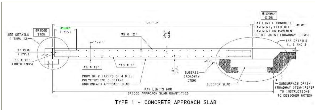
**Figure 68 PennDOT Concrete Approach Slab**
