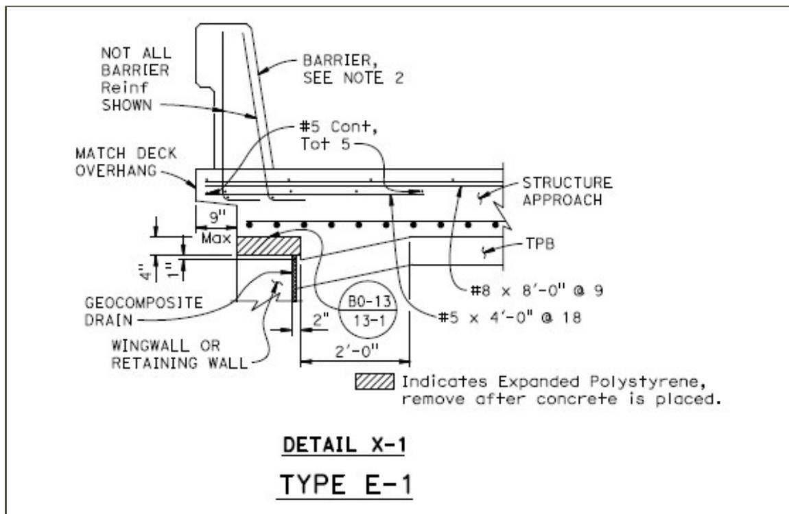
*Figure 87 Caltrans Barrier Rail (Caltrans Standard Plan B9-5)*
