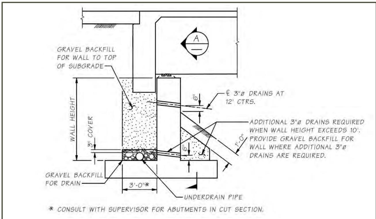
**Figure 50 WSDOT Drainage and Backfill Detail (BDM Fig. 7.5.11-1)**
