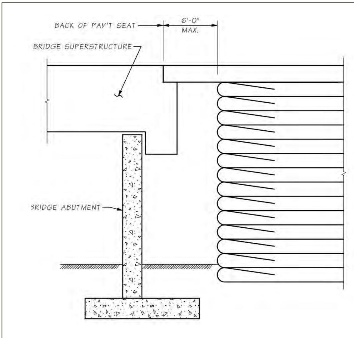
**Figure 99 WSDOT Isolated Abutment (BDM Fig 7.5.1-5)**
