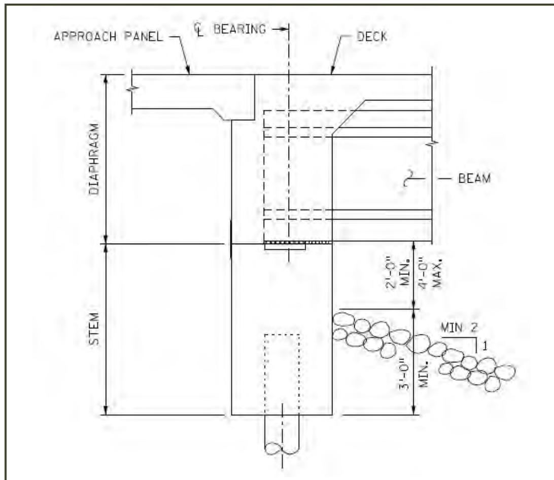
Figure 33 Integral Abutment Detail (courtesy MnDOT)
