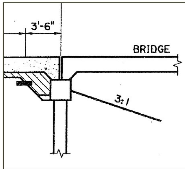
*Figure 57 LaDOTD Bridge / Abutment Interface*
