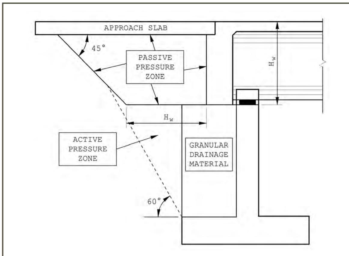
Figure 26 WSDOT Semi-Integral Abutment (WSDOT BDM Figure 4.2.11-1A)
