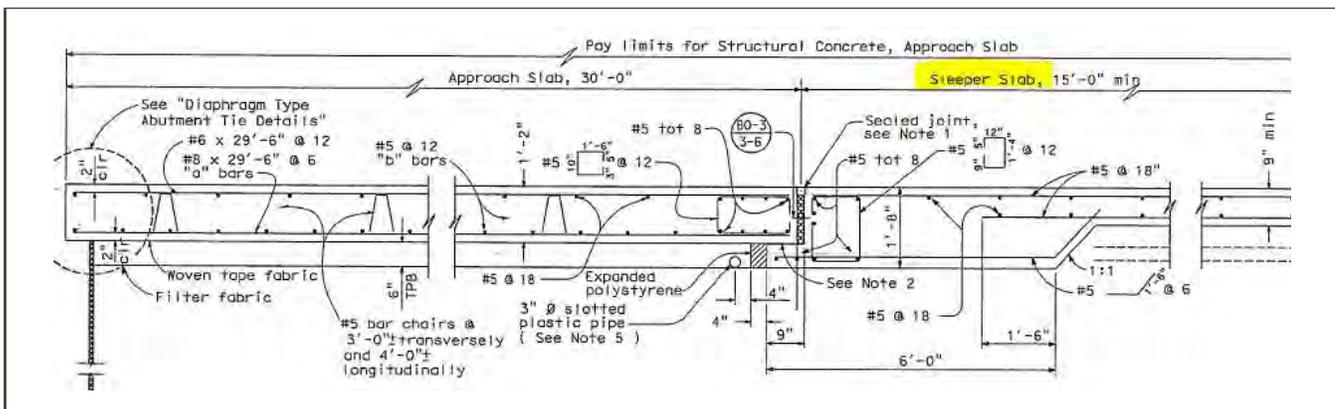
Figure 83 Caltrans Sleeper Slab Detail
