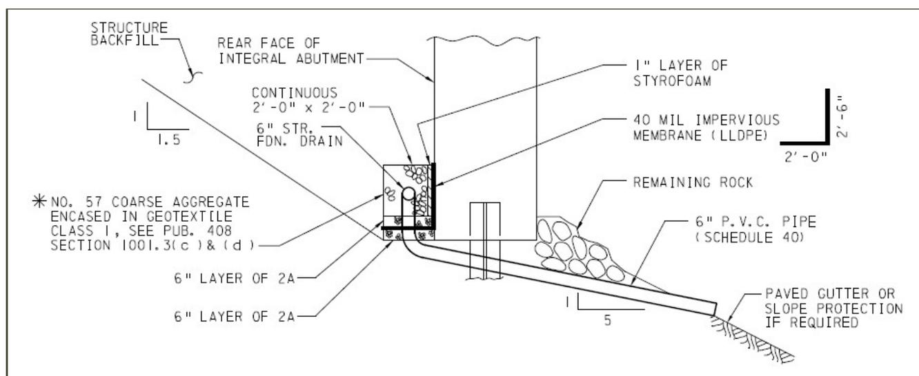
**Figure 101 PennDOT Enhanced Drainage Detail for Abutments without Approach Slab**
