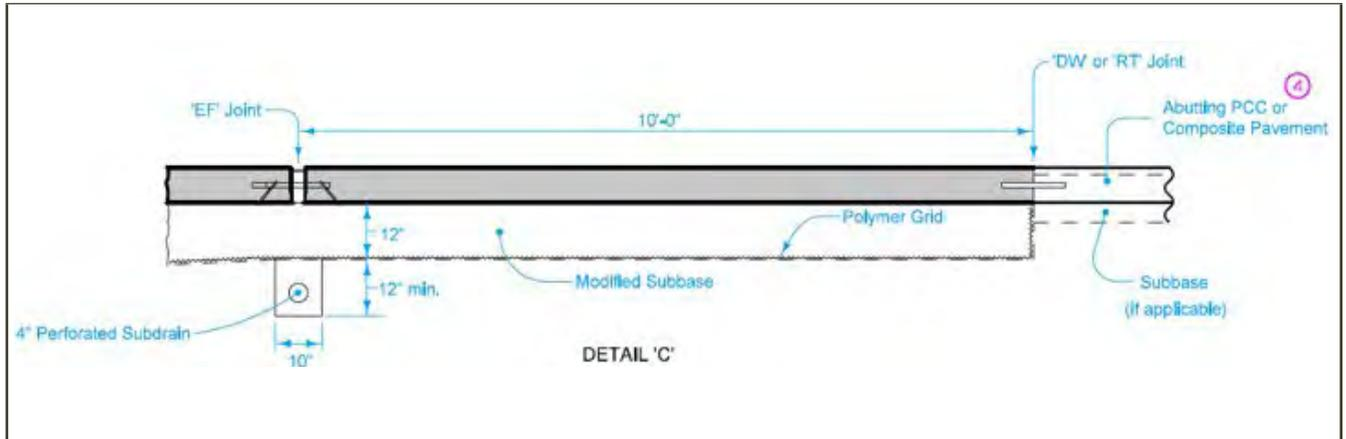
Figure 75 Iowa DOT Slab to Pavement Connection
