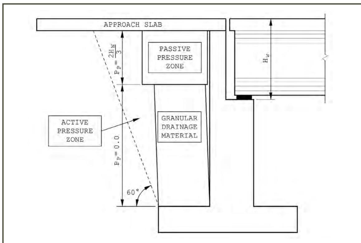
Figure 28 WSDOT L-Shape Abutment Backwall Does Not Fuse (WSDOT BDM Figure 4.2.11-1C)
