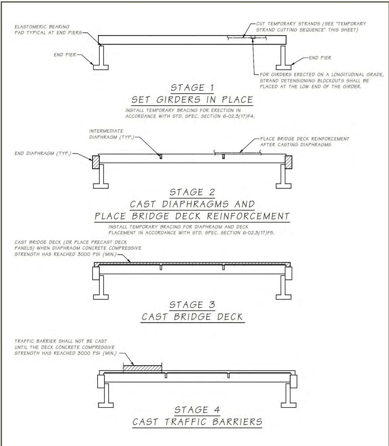
Figure 30 WSDOT Single Span Prestressed Girder Construction Sequence (WSDOT BSD 5.6-A2-1)
