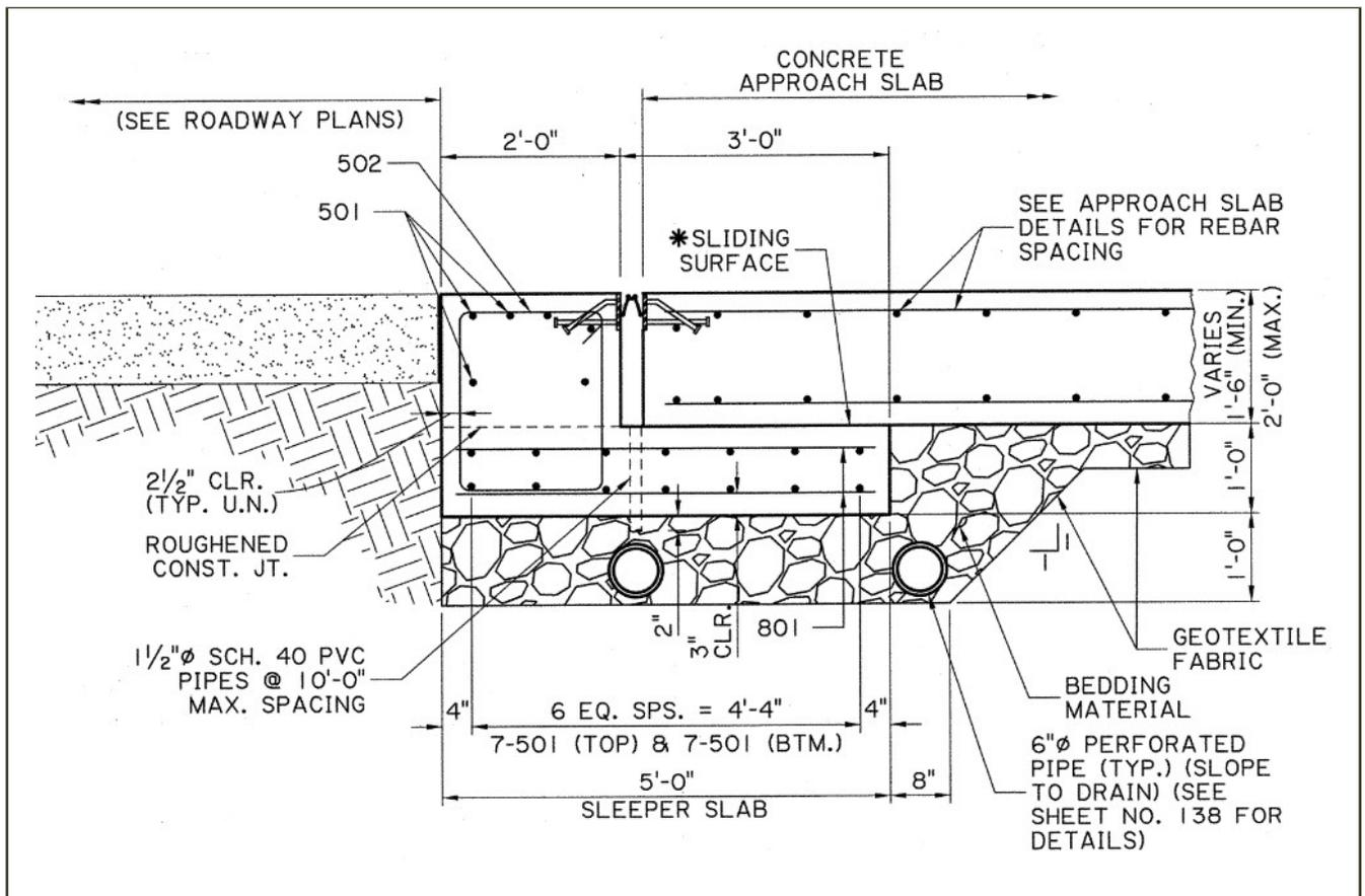
Figure 76 LaDOTD Slab to Pavement Connection
