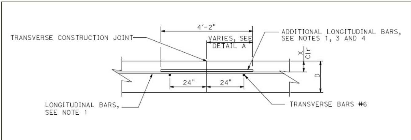
**Figure 73 Caltrans Detail at New Pavement (Caltrans Standard Plan P14)**
