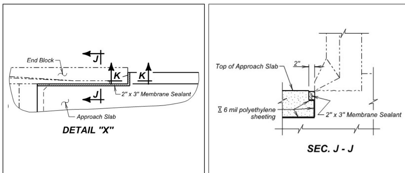
Figure 65 SDDOT Approach Slab/Wing Wall Detail
