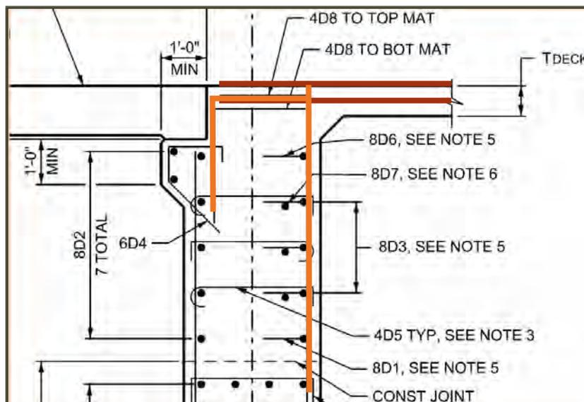
Figure 60 UDOT Bridge Deck to Backwall Details
