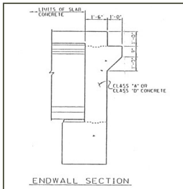
**Figure 43 TDOT Integral Endwall Section**
