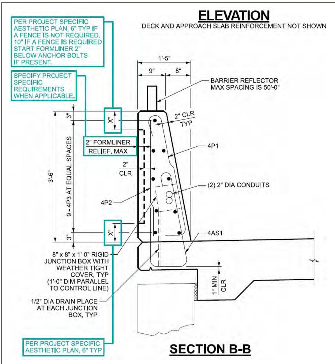
Figure 88 UDOT Barrier Rail
