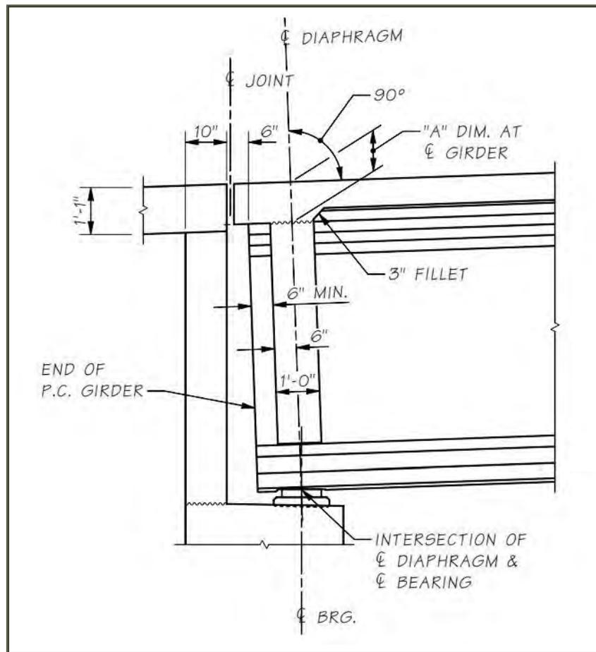
Figure 62 WSDOT L-Shaped End Pier (BDM Fig. 5.6.2-4)
