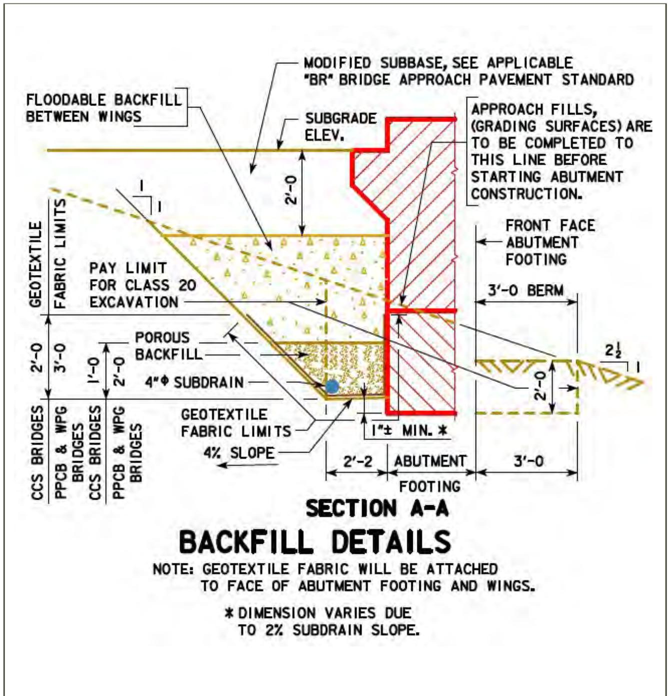
Figure 91 Iowa DOT Backfill Details
