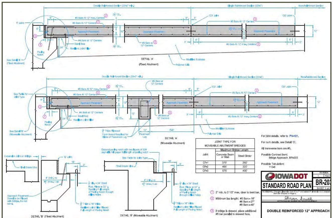
Figure 23 Iowa DOT Approach Slab Details
