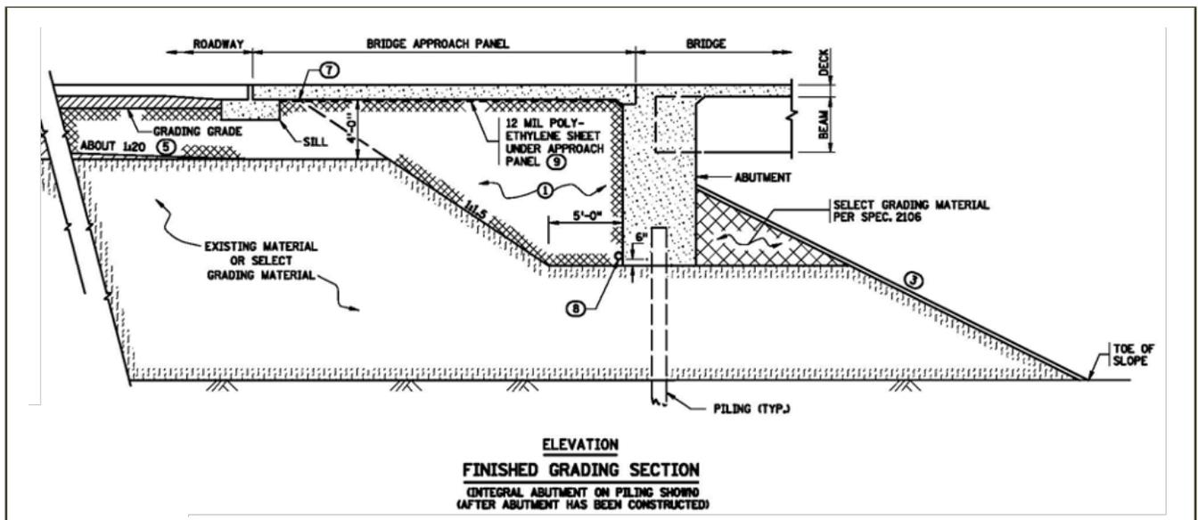
*Figure 94 MnDOT Finished Grading Section*
