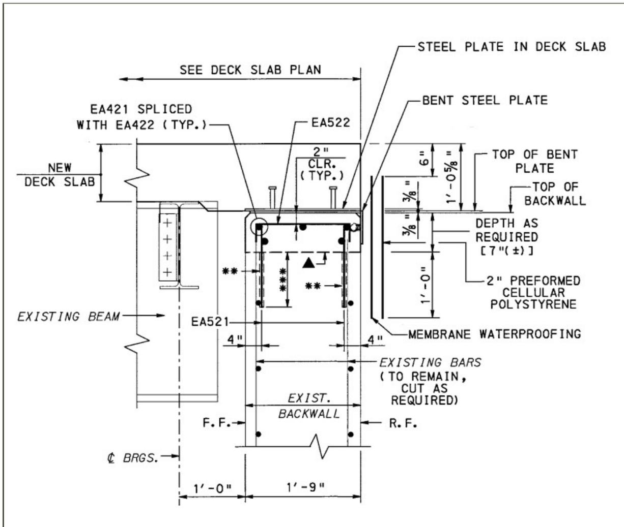
Figure 104 PennDOT Deck Extension/Eliminating Joints
