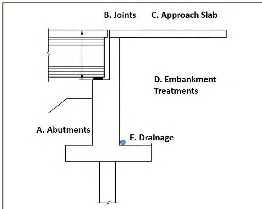
*Figure 32 General Bridge End Components*
