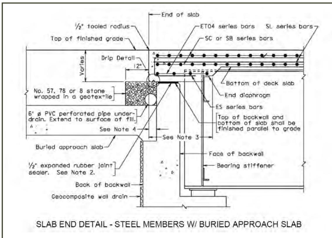
Figure 35 Slab Over Detail (Courtesy VDOT)
