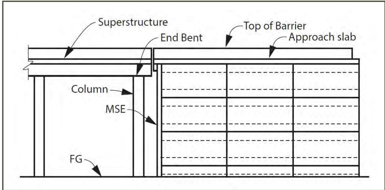
Figure 36 Caltrans End Bent with Isolated MSE on three sides
