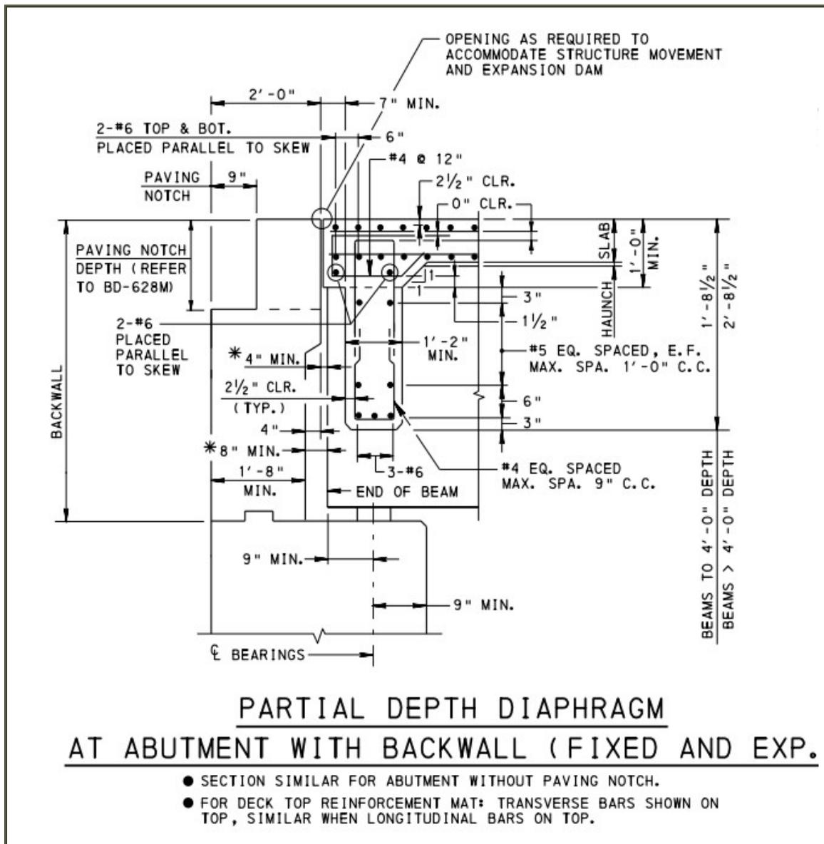
*Figure 58 PennDOT Diaphragm at Abutment (PennDOT BD656M)*
