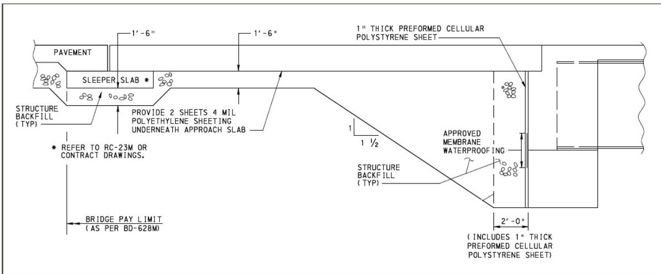
**Figure 95 PennDOT Structural Backfill**
