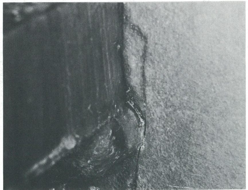
Figure 20. Typical surface crack at weld toe of web attachment.
