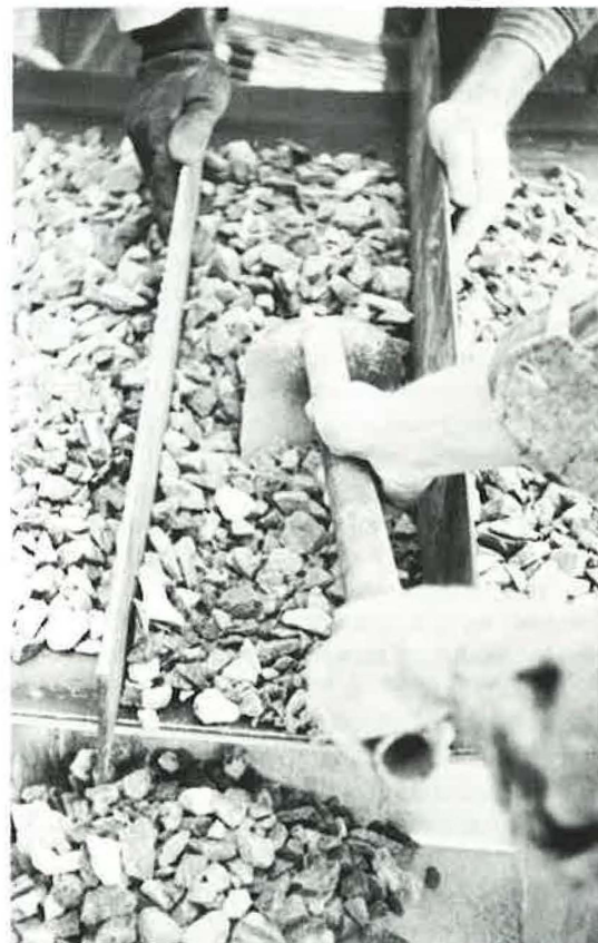
Figure 13. The belt sampling technique consisted of defining a specific belt area with the aid of metal templates, then removing all aggregate between the metal plates. Two test portions were removed each time the belt was stopped so that within-batch variance could be determined.
