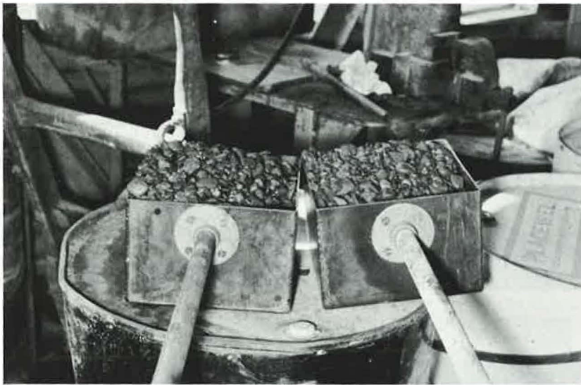
Figure 17. These sampling devices, used to cut the aggregate stream discharged into the weigh hopper in Series Nos. 7 and 8, are typical of those used to sample flowing streams of aggregate.
