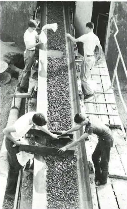
Figure 13. The belt sampling technique consisted of defining a specific belt area with the aid of metal templates, then removing all aggregate between the metal plates. Two test portions were removed each time the belt was stopped so that within-batch variance could be determined.
