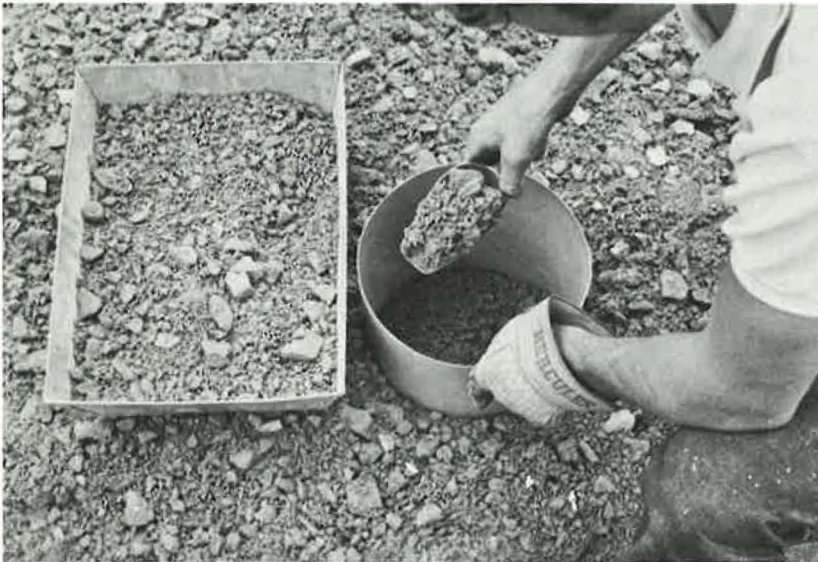
Figure 20. The roadway was sampled after the aggregate had been placed with a spreader and before compaction. A 10-in. diameter hoop defined the sampling areas and all material within the hoop was removed for testing.
