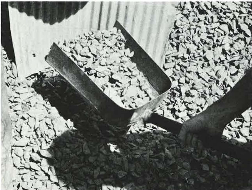
Figure 22. The modified shovel (lower photo) is generally recommended for hand sampling, particularly in the case of aggregates with a wide range of particle sizes. However, the narrow shovel (upper photo), a standard sampling tool used by some State highway departments, yielded identical results in the experimental sampling of the aggregate shown.
