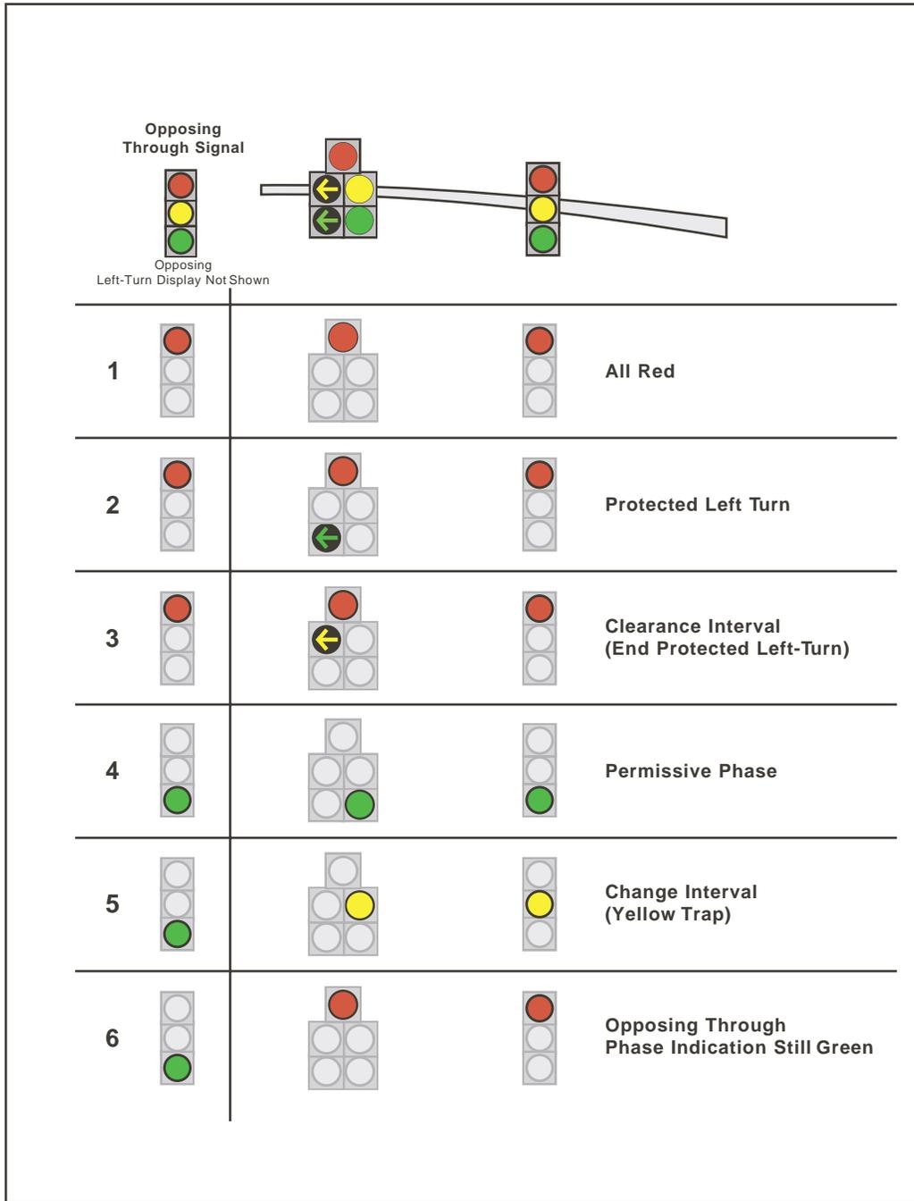
Figure 1-2. Yellow trap with MUTCD 5-section PPLT display.
