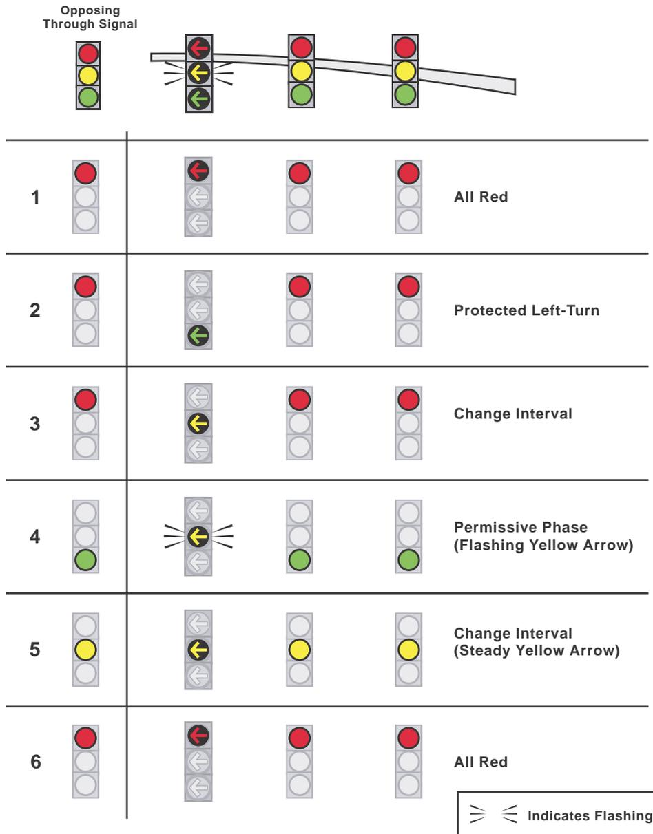
Figure 3-20. Operation of Jackson County, Oregon’s 3-section flashing yellow arrow PPLT display.
