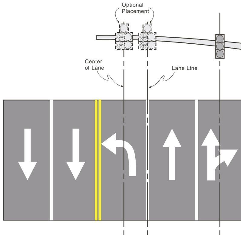
Figure 2-3. Overhead PPLT display placement options.
