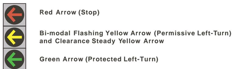
Figure 3-19. Jackson County, Oregon—3-section retrofit to flashing yellow arrow PPLT display.
