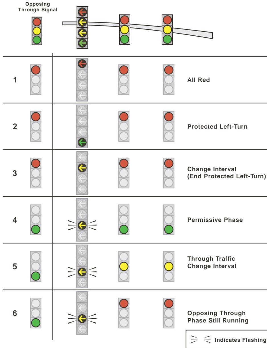
Figure 4-1. Flashing yellow arrow logical link.
