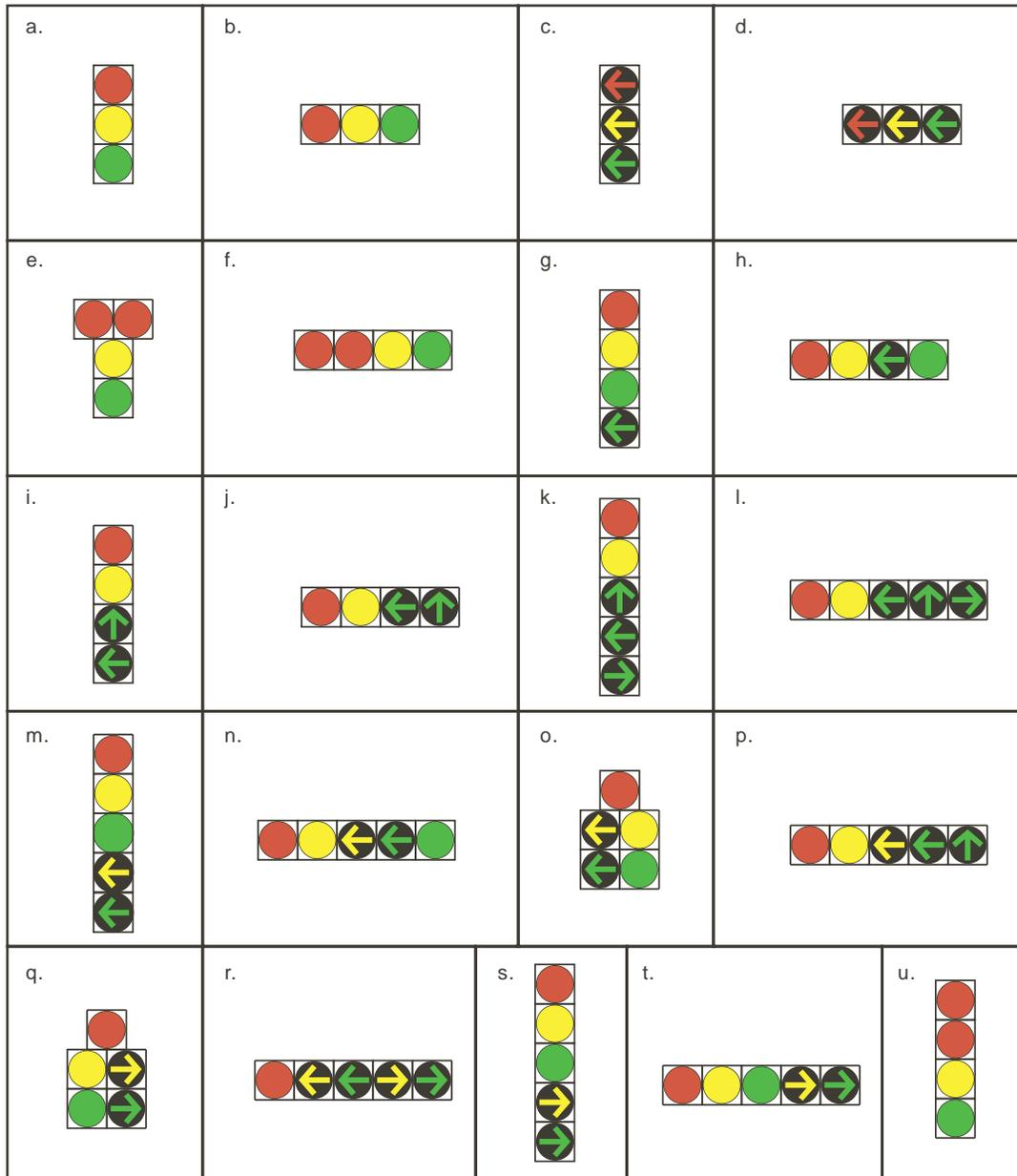
Figure 2-1. MUTCD arrangements of traffic signal displays.
