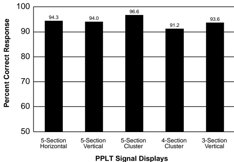
Figure 3-9. Driver understanding of all-red indications in PPLT signal displays.
