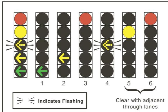
Figure 3-21. Broward County flashing yellow arrow display arrangement.
