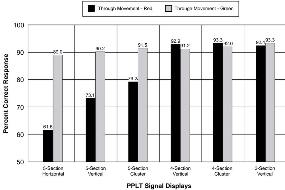
Figure 3-10. Driver understanding of protected indications in PPLT signal displays.
