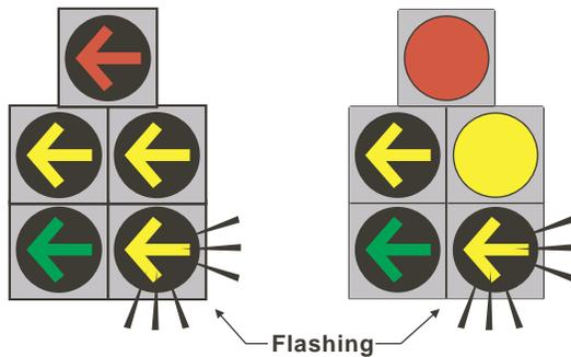
Figure 5-1. Potential flashing yellow arrow retrofit to five-section cluster display (exclusive left-turn display).
