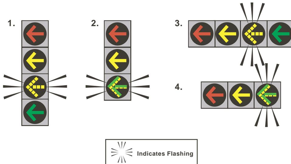
Figure 3-18. Exclusive flashing yellow arrow display faces.
