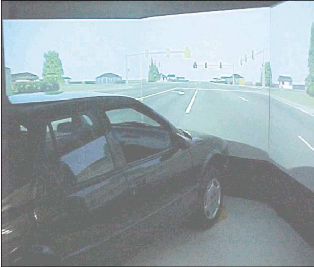
Figure 3-15. UMass Human Performance Laboratory driving simulator.
