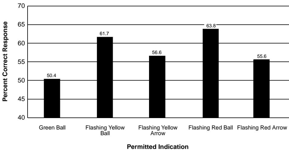
Figure 3-11. Percentage of correct responses for the permitted indications in PPLT signal displays.
