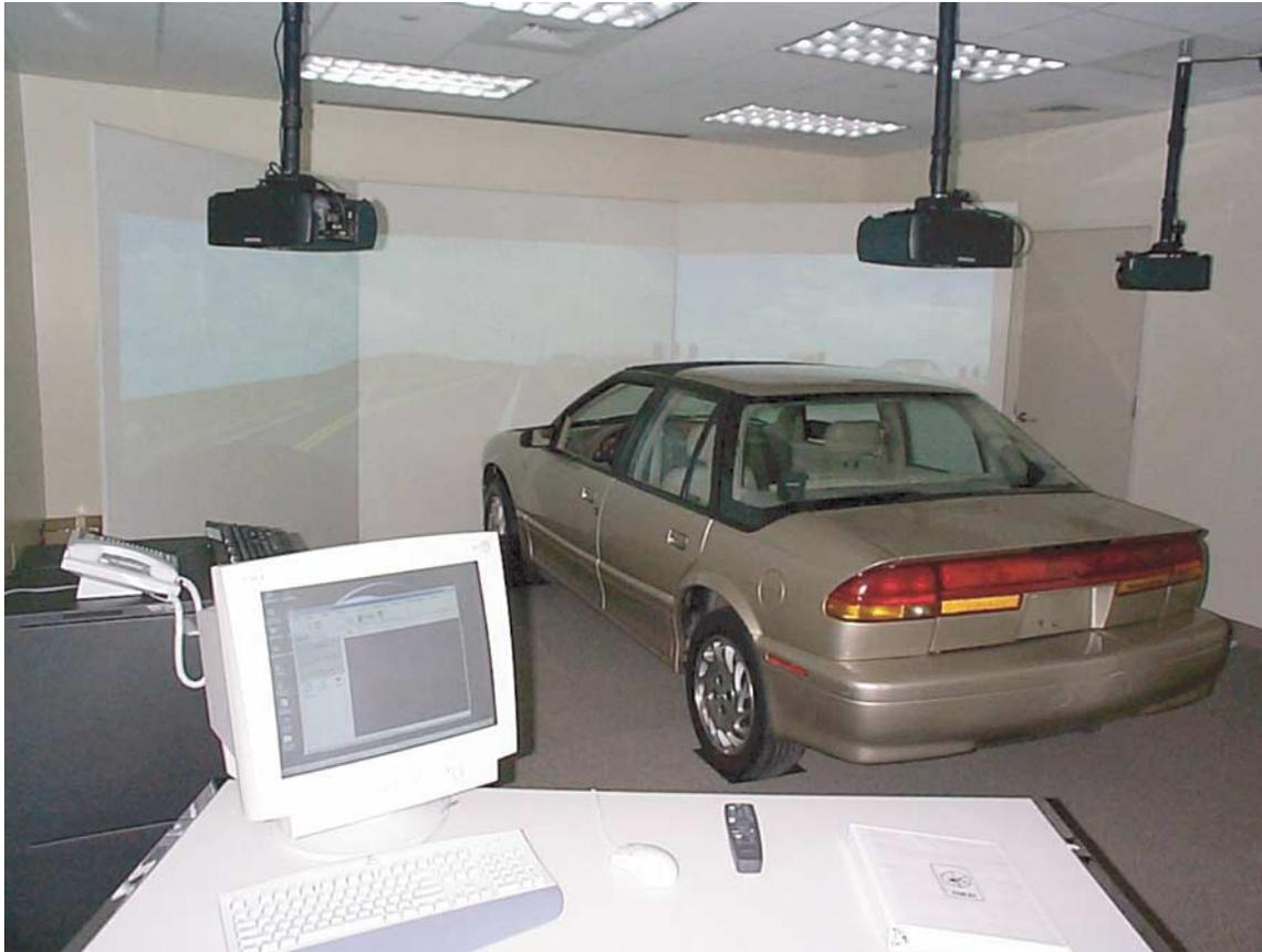
Figure 3-16. TTI driving environment simulator (DESi).
