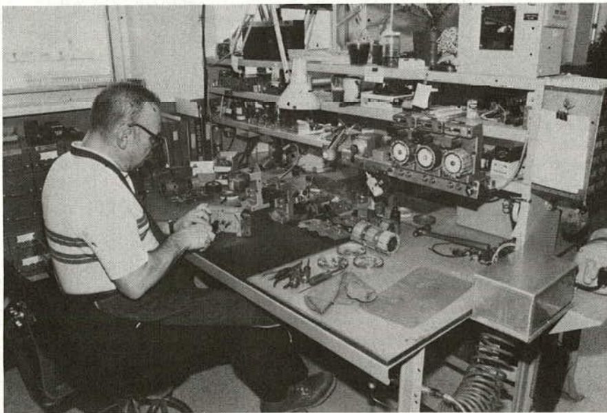
FIGURE 6 Electromechanical dial units are cleaned every 9 to 12 months at the City of Milwaukee signal shop.
