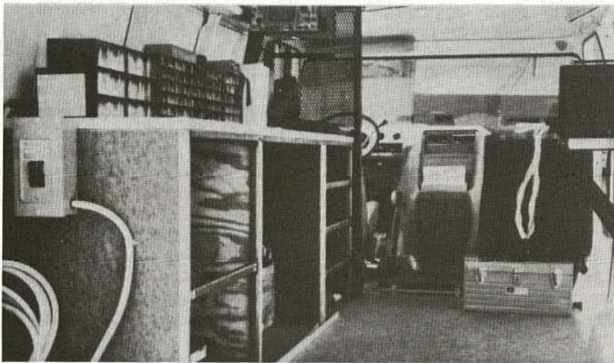
FIGURE 21 Shreveport's maintenance van carries testing devices, work benches, and spare parts (57).
