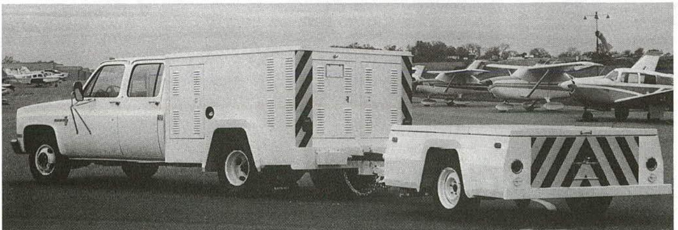
FIGURE 32 Locked wheel skid trailer (Cox and Sons Model 9000).
