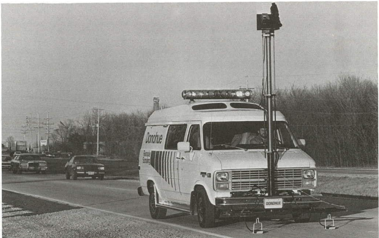
FIGURE 21 Remote sensing using infrared thermography and ground penetrating radar (Donohue and Assoc.).
