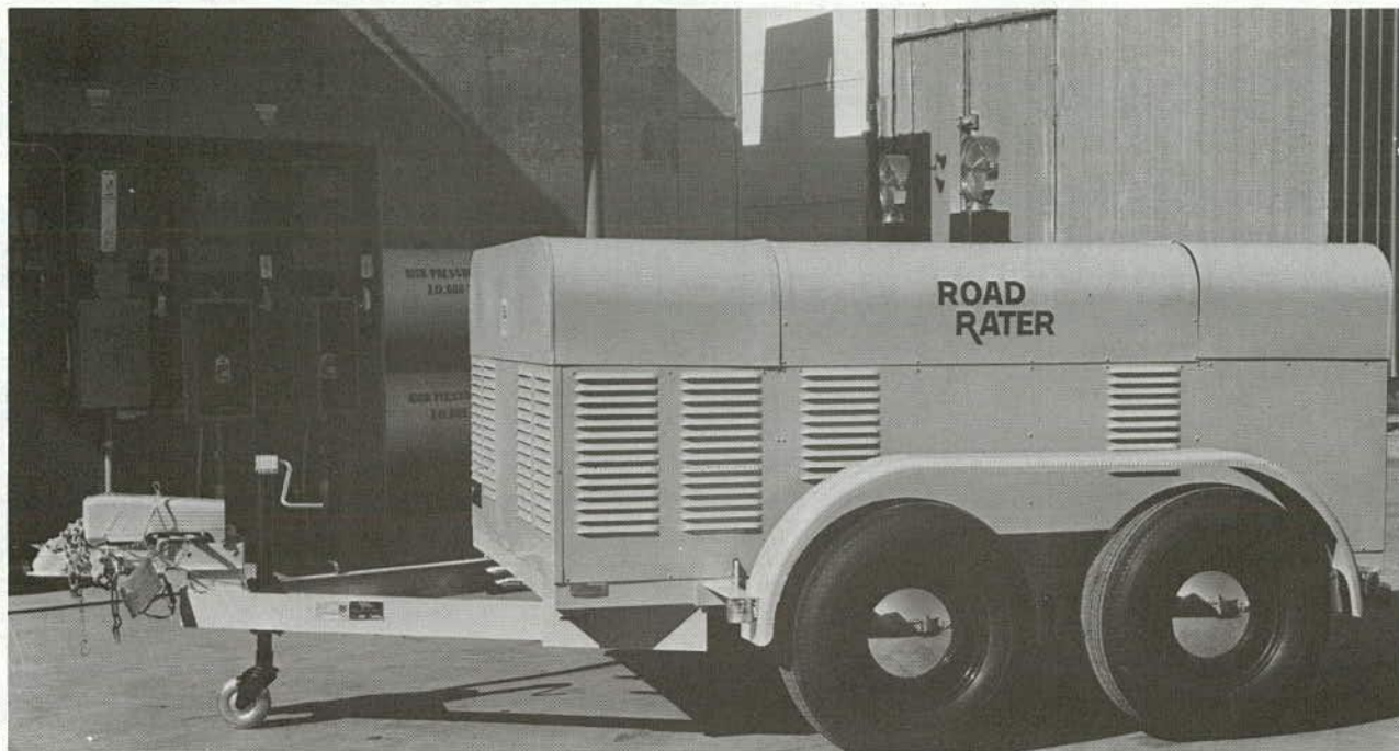
FIGURE 13 Model 400B trailer mounted Road Rater (Foundation Mechanics, Inc.). (Note that the model 400B can be van mounted.)
