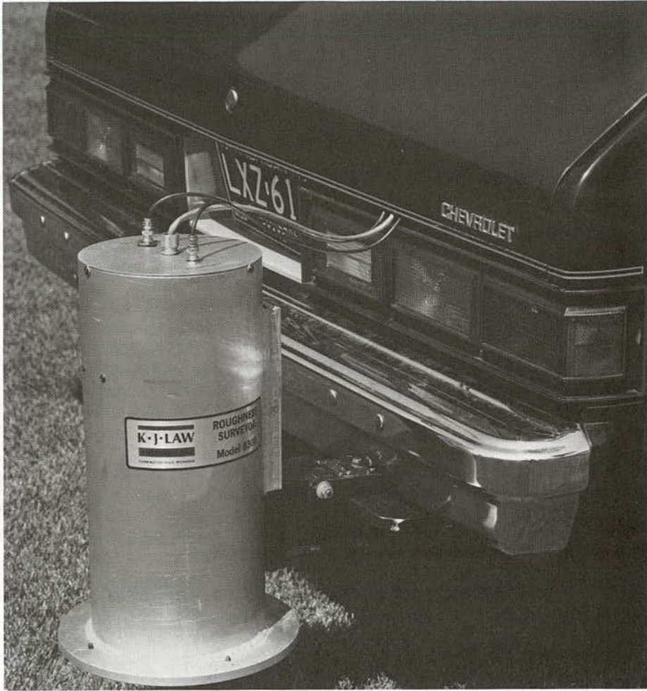
FIGURE 46 Ultrasonic displacement measurement cannister mounted on roughness measuring vehicle (K.J. Law Model 830V).
