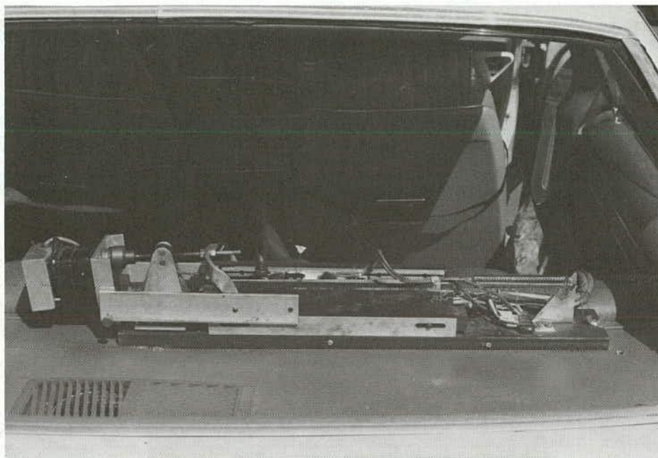
FIGURE 38 Looking into rear deck from outside of passenger vehicle (Shop made PCA Roadmeter).
