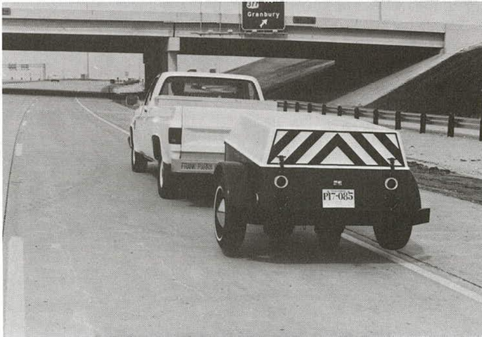
FIGURE 10 Dynaflect in operation (SIE, Inc.).
