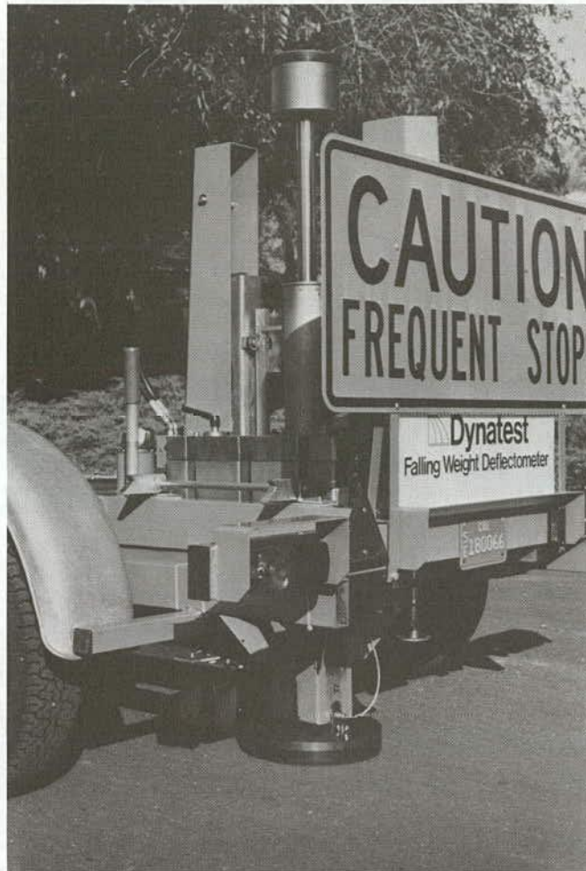
FIGURE 18 Falling-weight deflectometer in operating position (Dynatest Consulting, Inc., Model 8002).
