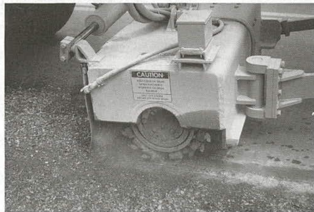
FIGURE 18 A medium-sized scarifier head.
