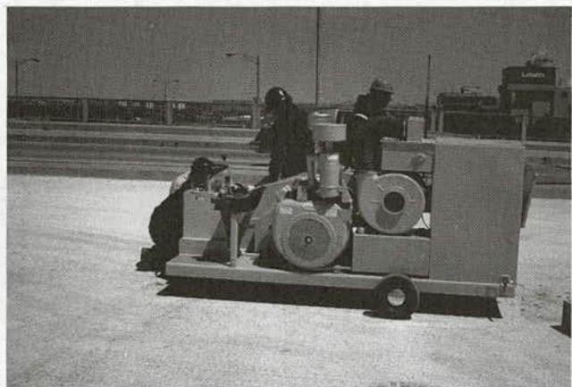
FIGURE 21 A commercial shotblasting machine.
