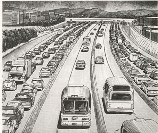
Barrier-separated facility being constructed along I-5 FIGURE A-7 Orange County HOV implementation.
