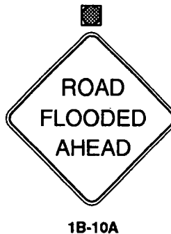
FIGURE 9 Water on roadway, active devices.
