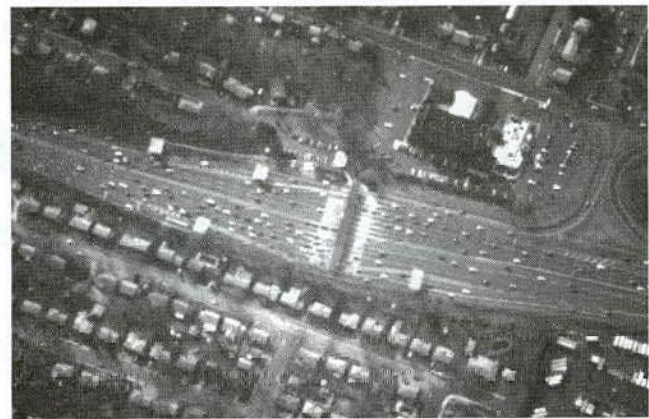
FIGURE 8 Branch toll lanes, Garden State Parkway Bergen toll plaza. Note the branch toll lanes both before and after the mainline toll plaza (New Jersey Highway Authority).
