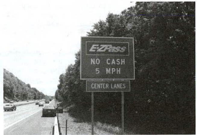
FIGURE 9b Electronic toll collection (ETC) lane advance sign, Spring Valley Toll Plaza, New York State Thruway (informs motorists on location of E-ZPass lanes).
