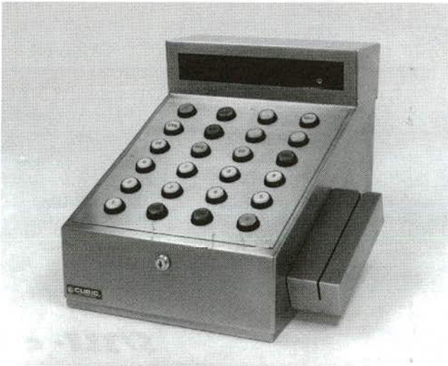
FIGURE 25a Toll collection terminal (TCT) with magnetic card swipe reader mounted on the right (Cubic Automatic Revenue Collection Group, San Diego, California).
