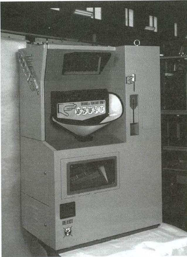
FIGURE 17a Automatic coin machine (ACM) with magnetic card swipe reader to be used on E-470 and by the Orlando-Orange County Florida Expressway Authority.
