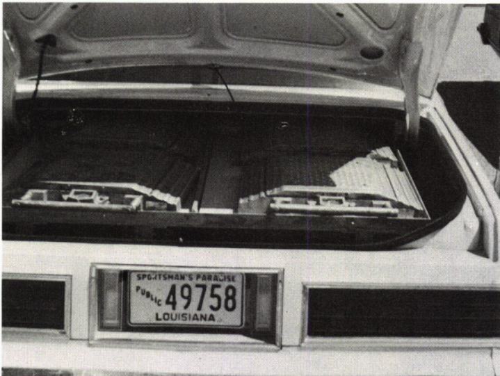
FIGURE 23 Methods of transporting portable scales. Top : Two portable scales and six wooden ramps transported by a station wagon in Arkansas. Bottom left : In Louisiana six scales (two scales are under the four visible scales) are carried in the truck of a patrol car. Bottom right : In Maryland portable scales are transported in a pickup truck. Note that the left rack is turned over the tailgate for easy handling. The rack on the right is in the transport position.
