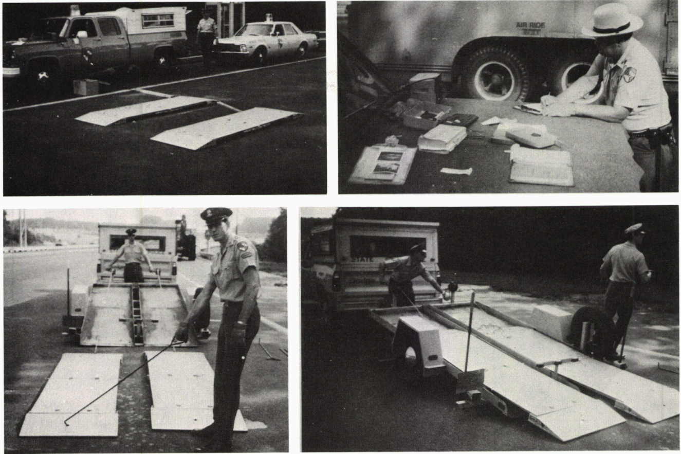
FIGURE 24 Top left: A 7-ft (2.1-m) semiportable scale set up for operation. Note the steel channels used to protect the cables. Top right: The enforcement officer reads the weight on the digital readout using the hood of the pickup truck. Bottom: The tilt trailer used in Maryland to transport the semiportable scales differs from the trailer suggested by the manufacturer. The two boat winches pull the scales onto the trailer.
