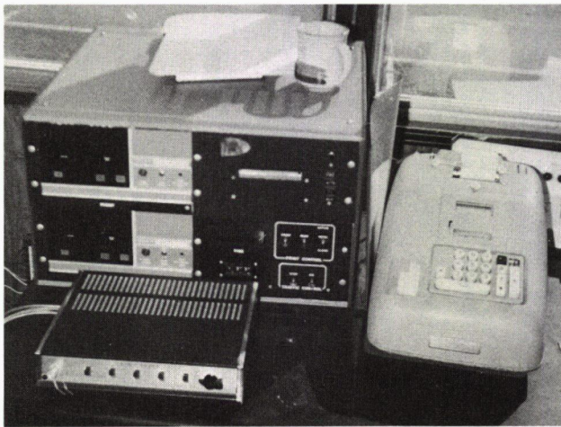
FIGURE 11 Semiportable scales used at a permanent weigh station on Interstate Route I-75 near Macon, Georgia. The digital readout is transferred to the adding machine by the enforcement officer and totaled for gross weight.
