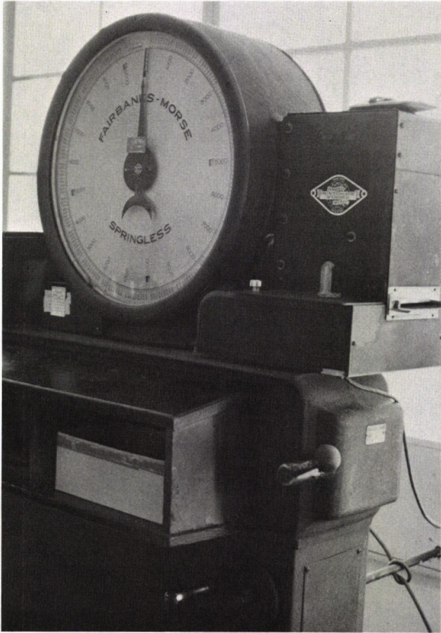
FIGURE 9 Single-platform beam scale. The dial is visible to both the enforcing officer and the truck driver (see Figure 8, bottom).
