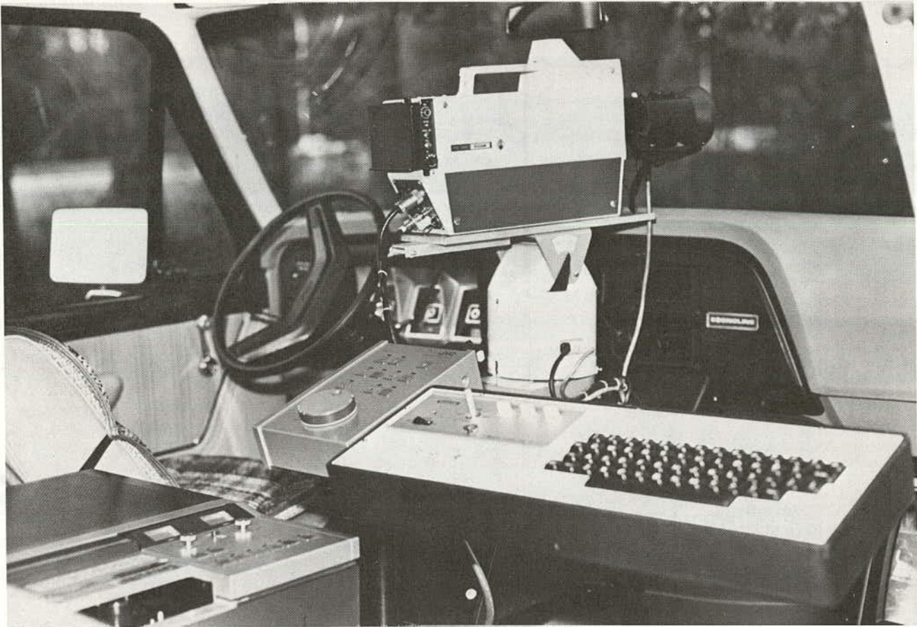
FIGURE 28 Videologging camera and equipment (Travel Technology Corp.).
