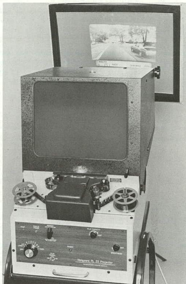
FIGURE 15 Wall projection from a stop-motion analyzer (Vanguard Instrument Corp.).
