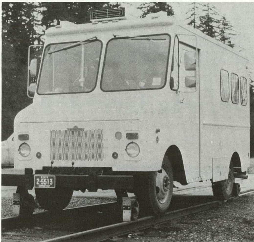
FIGURE 27 Photolog van for use on railroad tracks as well as on highways.
