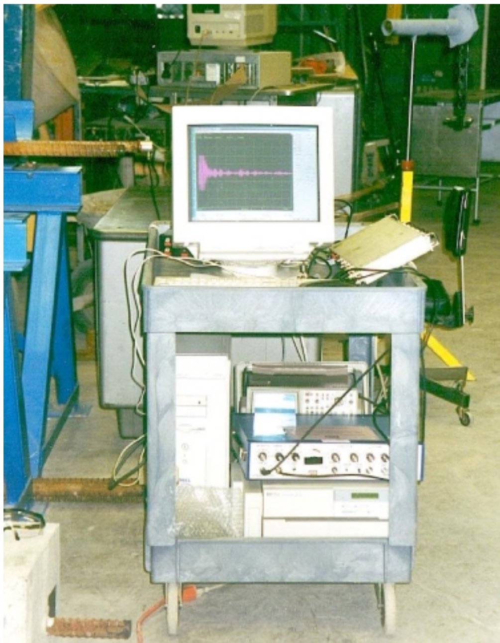
Figure 3-8. Computerized Data Acquisition System Placed on Cart.
