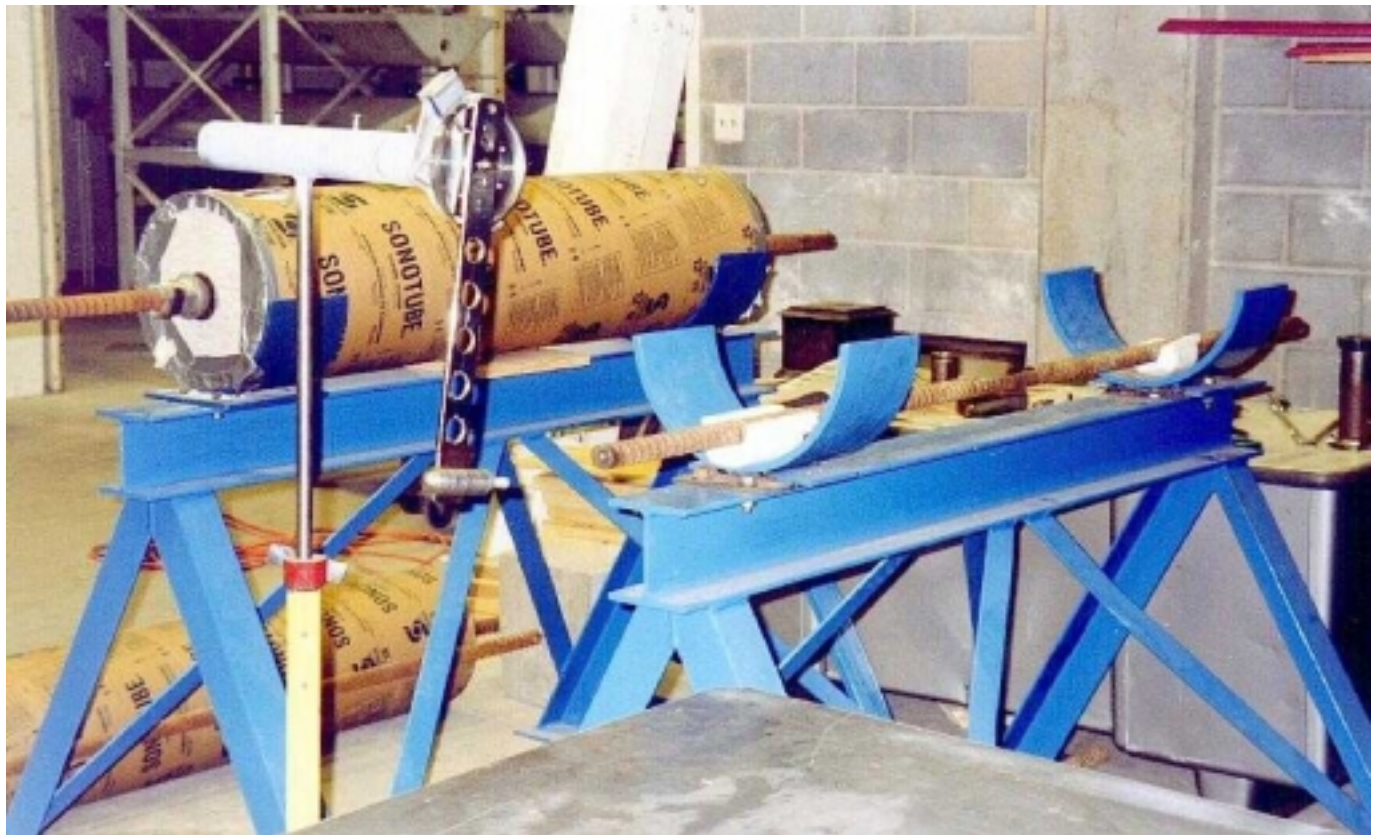
Figure 3-9: In-House Manufactured Pendulum With Ball Peen Hammer.
