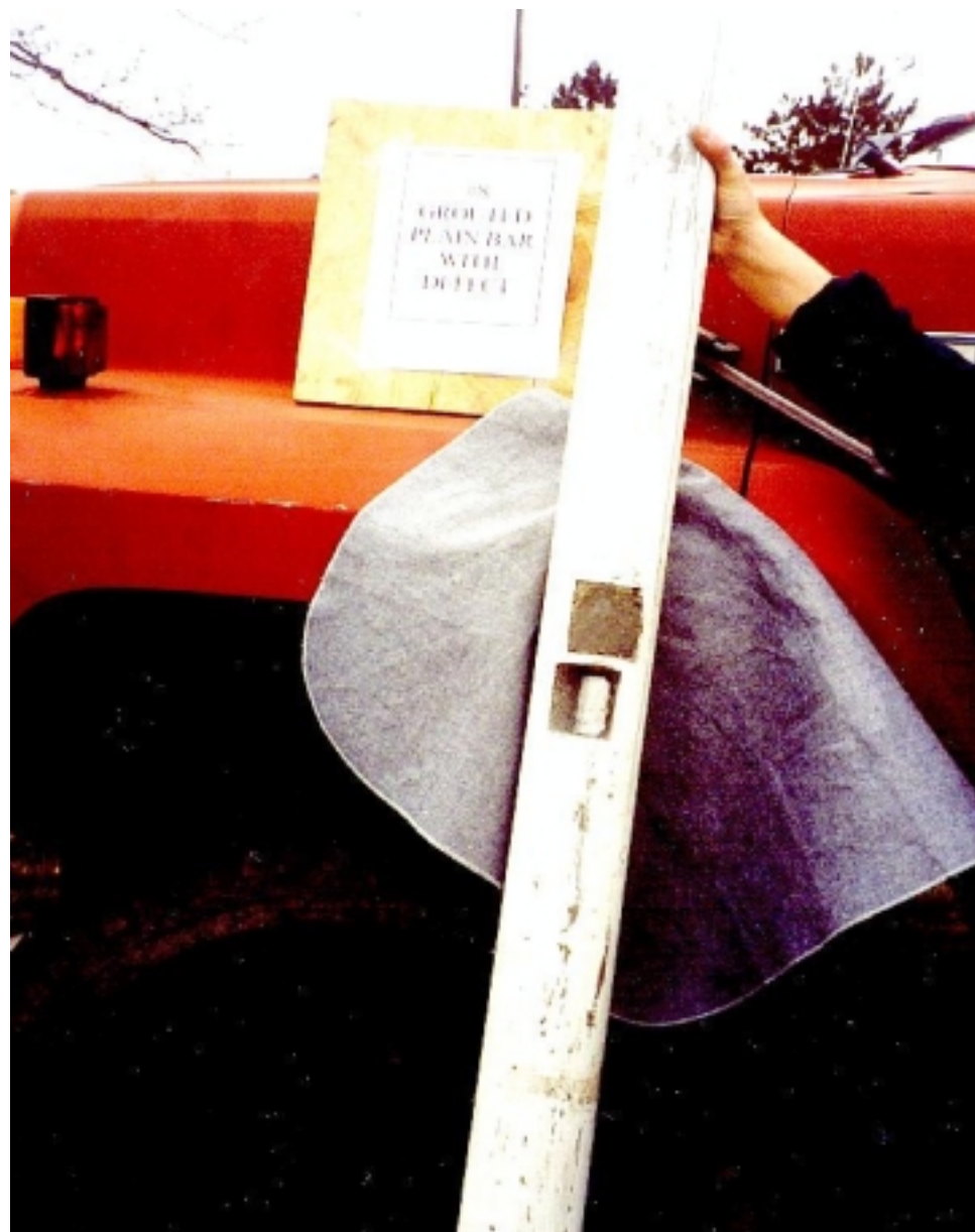
Figure 3-6(e): In-Situ Specimen #8: Grouted Bar With Defect.
