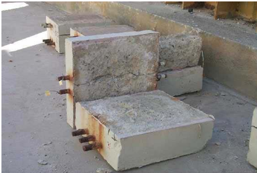
Figure A-5: Photograph of specimen after breaking apart along the lift line.
