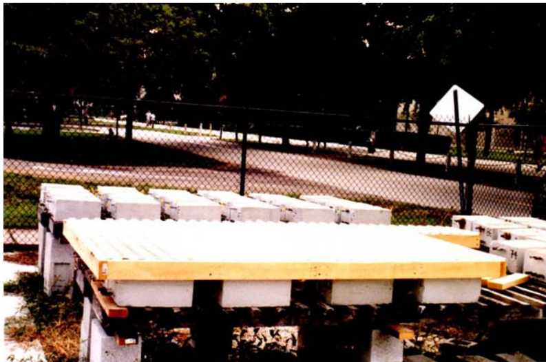
Figure A-2: Photograph of specimens under exposure. The plastic cover is to protect cyclically ponded specimens from rain.
