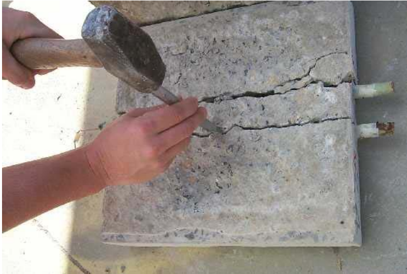
Figure A-6: Photograph of the upper lift containing two ECRs being broken open.
