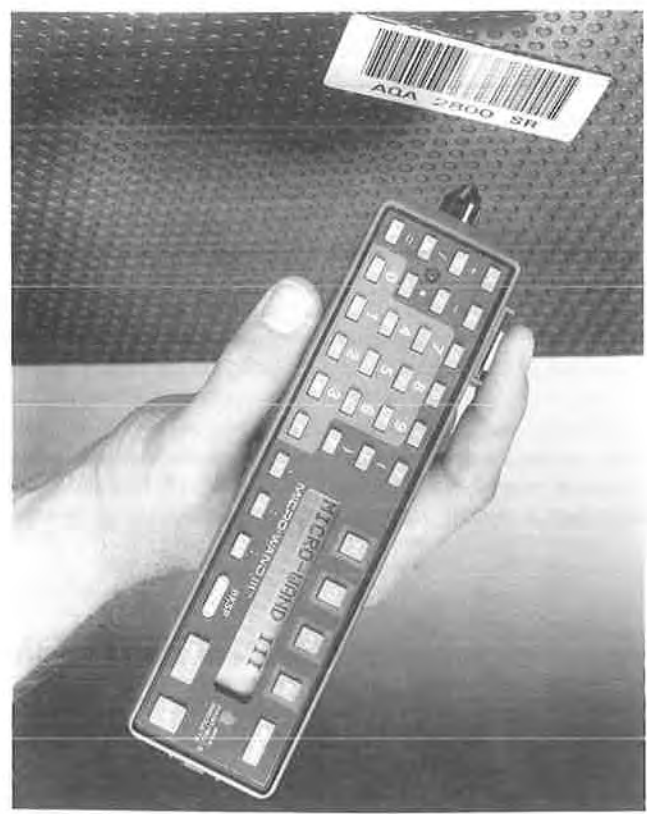
FIGURE 5. Micro-Wand III Hand-Held Entry Device (Micro-Wand III is a registered trademark of Hand Held Products, Inc.)
