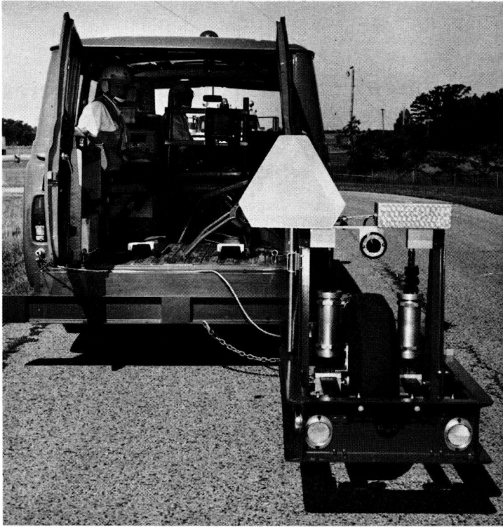
Figure 1. BPR-type, road roughness indicator, Model CT-444.
