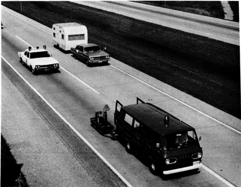
Figure 2. Roghometer test wheel is towed in the outside lane to record most severe condition.
