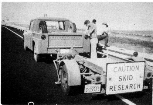
Figure 6. Tow vehicle and skid trailer.
