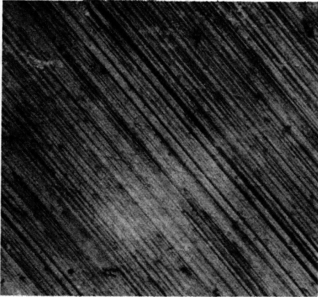
(i) \text{CaCO}_3 (c) by \text{Al}_2\text{O}_3 Abrasive
