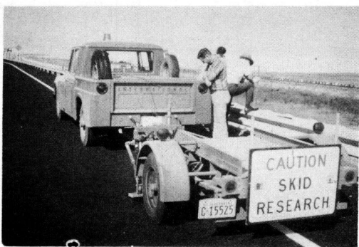
Figure 6. Tow vehicle and skid trailer.
