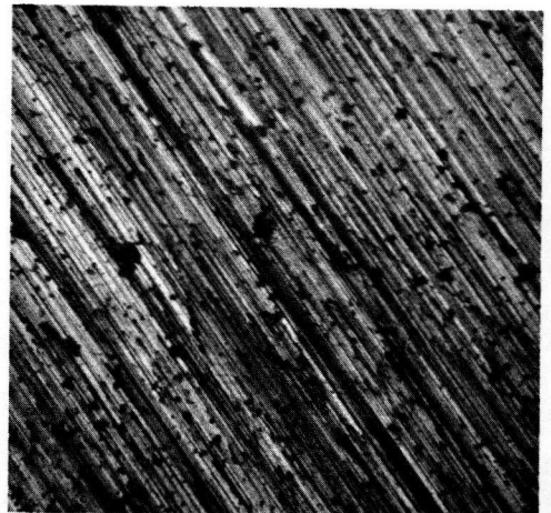
(f) \text{CaCO}_3 (c) by \text{SiO}_2 Abrasive
