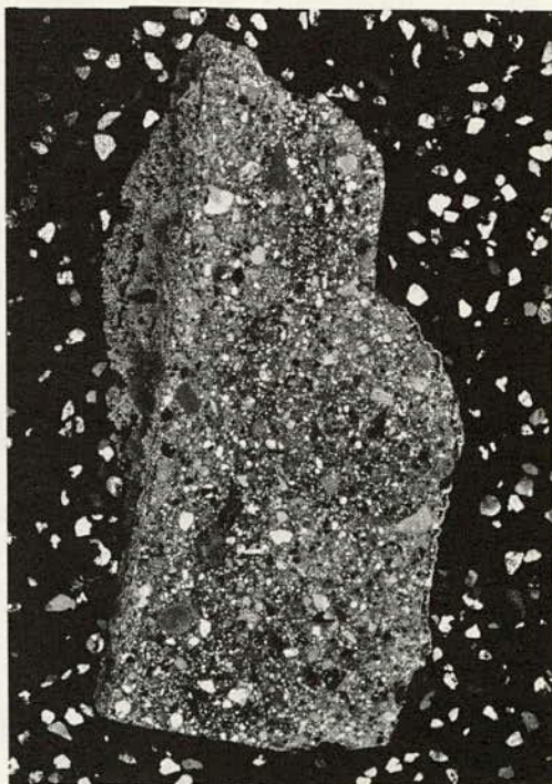
Figure 3. Total photo of a thin section prepared from a deteriorated piece of concrete taken from the outside upper part of a chimney (crossed nicols, 1.26x magnification).
