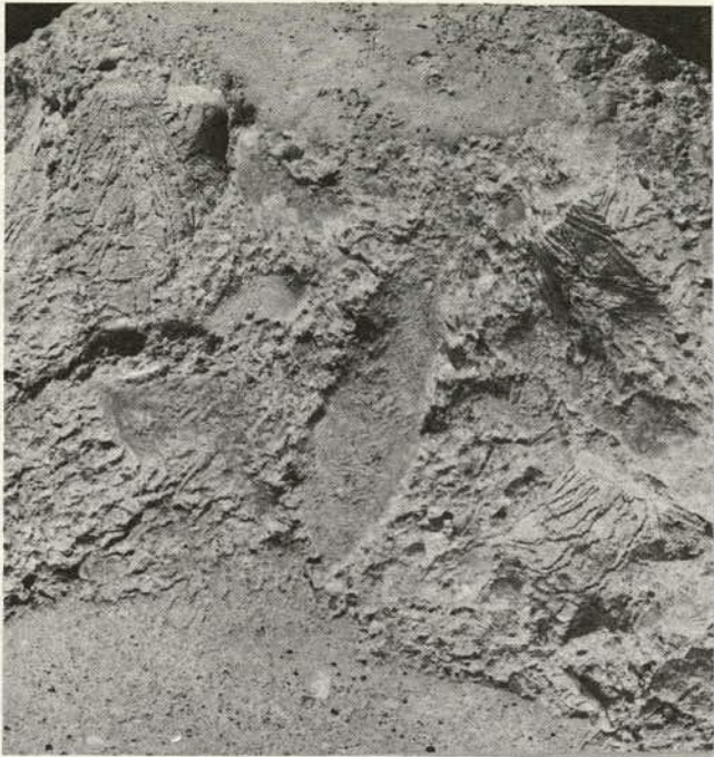
Figure 1. Formerly present ice crystals were responsible for the patterned imprints in aggregate sockets (magnification 1.8X).
