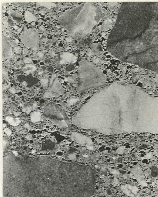
Figure 5. Magnified portion of the central area shown in Figure 4. The air content was determined to be 15 percent (magnification 3X).
