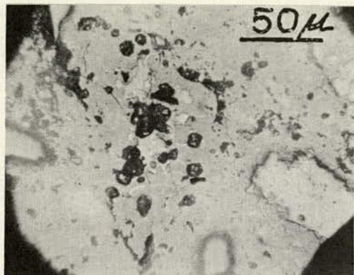
Figure 17. Polished section that shows residual and relic cement particles and microcracking.
