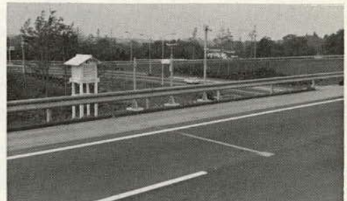
Figure 3. Road surface moisture meter.
