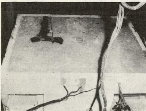
Figure 1. Top view of laboratory slab installed in cold room.
