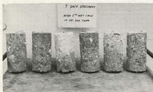
Figure 11. Condition of 7-sack concrete after 5 and 6 cycles of alternate immersion in sodium formate.
