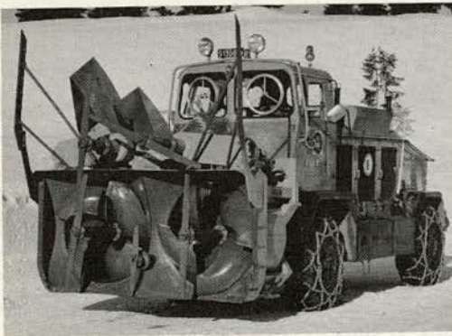
Figure 8. Snow-removing machine with clearing height up to 3.5 m and clearing width of 2.9 m.
