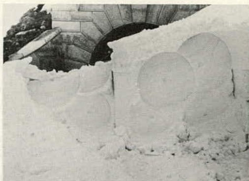
Figure 10. Cleared road with clearing profiles in hard snow (snow depth 3.5 m).
