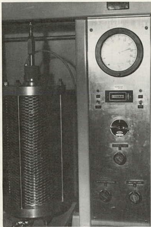
Figure 7. Repeated-loading apparatus with triaxial cell in place in left bay.
